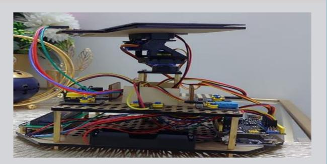
After uploading the test code and powering it up, the servos rotate to the initial angle. And when the ambient light sensor detects changes in light intensity, servos rotate to the position where the light is the strongest and LCD1602 shows the value of the light intensity and temperature and humidity detected by the BH1750 and XHT11 respectively.
