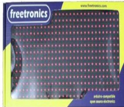
LED Dot Matrix Display Panel 32x16 (512 LEDs)
