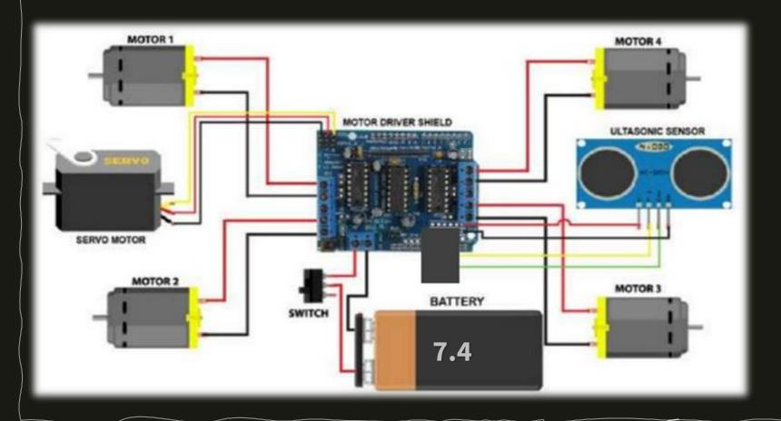
The Servo Motor is responsible for moving the Ultrasonic Sensor which is the main part of this project, then comes the four DC Motors which is responsible for moving the Robot Car, then we have the Power Source (7.4) which is provided by two li-ion batteries of (3.7) which is connected to a Switch to control the power Motor Driver Shield connects all the parts together with the Arduino UNO and its main object is to control the movement of the motors.
