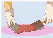
Once gel is foamed, use scoop and scraper to remove the congealed spill.
