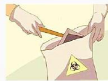
Place scoop, contents and scraper into bio hazard bag.
