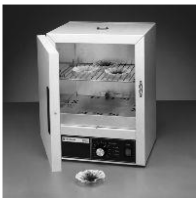
Conventional laboratory oven used for drying materials.
