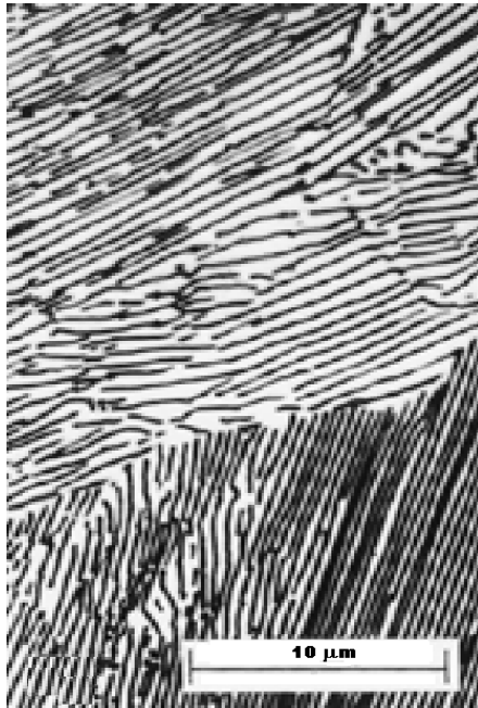
Near eutectoid temperature Slow diffusion => coarse pearlite
