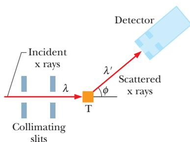
**Fig. 38-3** Compton's apparatus. A beam of x rays of wavelength  $\lambda = 71.1$  pm is directed onto a carbon target T. The x rays scattered from the target are observed at various angles  $\phi$  to the direction of the incident beam. The detector measures both the intensity of the scattered x rays and their wavelength.
