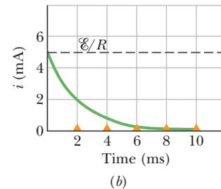
**Fig. 27-16** (a) A plot of Eq. 27-33, which shows the buildup of charge on the capacitor of Fig. 27-15. (b) A plot of Eq. 27-34, which shows the decline of the charging current in the circuit of Fig. 27-15. The curves are plotted for  $R = 2000 \Omega$ ,  $C = 1 \mu\text{F}$ , and  $\mathcal{E} = 10 \text{ V}$ ; the small triangles represent successive intervals of one time constant  $\tau$ .
