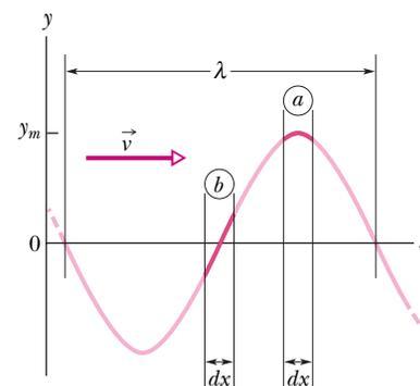
**Fig. 16-9** A snapshot of a traveling wave on a string at time  $t = 0$ . String element  $a$  is at displacement  $y = y_m$ , and string element  $b$  is at displacement  $y = 0$ . The kinetic energy of the string element at each position depends on the transverse velocity of the element. The potential energy depends on the amount by which the string element is stretched as the wave passes through it.
