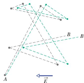
**Fig. 26-12** The gray lines show an electron moving from  $A$  to  $B$ , making six collisions en route. The green lines show what the electron's path might be in the presence of an applied electric field  $\vec{E}$ . Note the steady drift in the direction of  $-\vec{E}$ . (Actually, the green lines should be slightly curved, to represent the parabolic paths followed by the electrons between collisions, under the influence of an electric field.)
