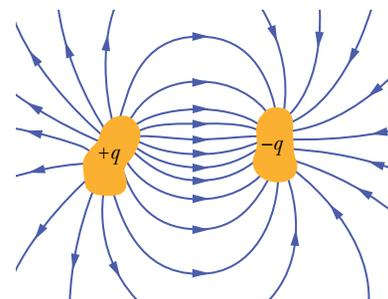
Fig. 25-2 Two conductors, isolated electrically from each other and from their surroundings, form a *capacitor*. When the capacitor is charged, the charges on the conductors, or *plates* as they are called, have the same magnitude  $q$  but opposite signs. (Paul Silvermann/Fundamental Photographs)
