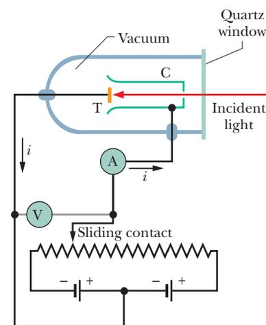
**Fig. 38-1** An apparatus used to study the photoelectric effect. The incident light shines on target T, ejecting electrons, which are collected by collector cup C. The electrons move in the circuit in a direction opposite the conventional current arrows. The batteries and the variable resistor are used to produce and adjust the electric potential difference between T and C.
