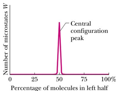
**Fig. 20-18** For a *large* number of molecules in a box, a plot of the number of microstates that require various percentages of the molecules to be in the left half of the box. Nearly all the microstates correspond to an approximately equal sharing of the molecules between the two halves of the box; those microstates form the *central configuration peak* on the plot. For  $N \approx 10^{22}$ , the central configuration peak is much too narrow to be drawn on this plot.
