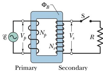
**Fig. 31-18** An ideal transformer (two coils wound on an iron core) in a basic transformer circuit. An ac generator produces current in the coil at the left (the *primary*). The coil at the right (the *secondary*) is connected to the resistive load  $R$  when switch  $S$  is closed.
