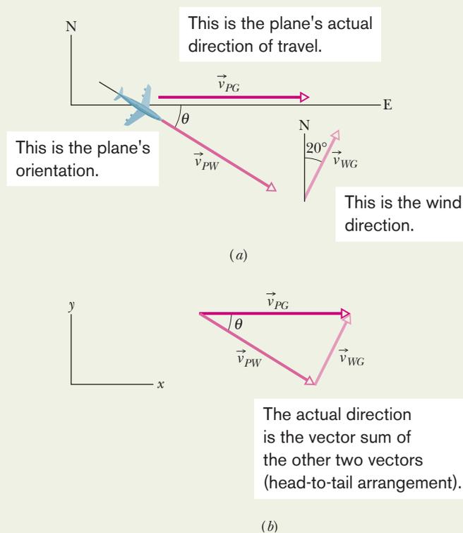
Fig. 4-20 A plane flying in a wind.
