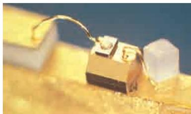
**Fig. 41-18** A junction laser developed at the AT&T Bell Laboratories. The cube at the right is a grain of salt. (Courtesy AT&T Archives and History Center, Warren, NJ)
