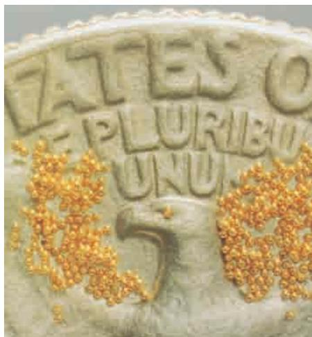
**Fig. 43-13** The small spheres on the quarter are deuterium–tritium fuel pellets, designed to be used in a laser fusion chamber. (Courtesy Los Alamos National Laboratory, New Mexico)
