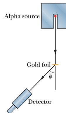
**Fig. 42-1** An arrangement (top view) used in Rutherford's laboratory in 1911–1913 to study the scattering of  $\alpha$  particles by thin metal foils. The detector can be rotated to various values of the scattering angle  $\phi$ . The alpha source was radon gas, a decay product of radium. With this simple “tabletop” apparatus, the atomic nucleus was discovered.
