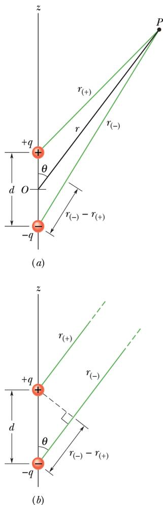
**Fig. 24-10** (a) Point  $P$  is a distance  $r$  from the midpoint  $O$  of a dipole. The line  $OP$  makes an angle  $\theta$  with the dipole axis. (b) If  $P$  is far from the dipole, the lines of lengths  $r_{(+)}$  and  $r_{(-)}$  are approximately parallel to the line of length  $r$ , and the dashed black line is approximately perpendicular to the line of length  $r_{(-)}$ .
