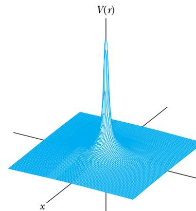
**Fig. 24-7** A computer-generated plot of the electric potential  $V(r)$  due to a positive point charge located at the origin of an  $xy$  plane. The potentials at points in the  $xy$  plane are plotted vertically. (Curved lines have been added to help you visualize the plot.) The infinite value of  $V$  predicted by Eq. 24-26 for  $r = 0$  is not plotted.
