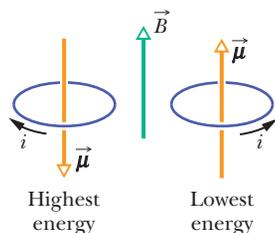
**Fig. 28-20** The orientations of highest and lowest energy of a magnetic dipole (here a coil carrying current) in an external magnetic field  $\vec{B}$ . The direction of the magnetic dipole moment  $\vec{\mu}$  via the right-hand rule shown for  $\vec{n}$  in Fig. 28-19b.
