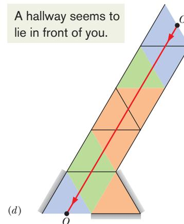
**Fig. 34-7** (a) Overhead view of a mirror maze. A ray from mirror  $B$  reaches you at  $O$  by reflecting from mirror  $A$ . (b) Mirror  $B$  appears to be behind  $A$ . (c) The ray reaching you comes from you. (d) You see a virtual image of yourself at the end of an apparent hallway.
