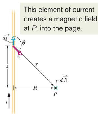
**Fig. 29-5** Calculating the magnetic field produced by a current  $i$  in a long straight wire. The field  $d\vec{B}$  at  $P$  associated with the current-length element  $i d\vec{s}$  is directed into the page, as shown.
