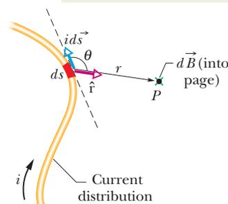
**Fig. 29-1** A current-length element  $i d\vec{s}$  produces a differential magnetic field  $d\vec{B}$  at point  $P$ . The green  $\times$  (the tail of an arrow) at the dot for point  $P$  indicates that  $d\vec{B}$  is directed *into* the page there.
