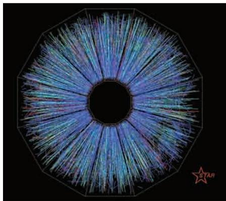
The violent head-on collision of two 30 GeV beams of gold atoms in the RHIC accelerator at the Brookhaven National Laboratory. In the moment of collision, a gas of individual quarks and gluons was created. (Courtesy Brookhaven National Laboratory)
