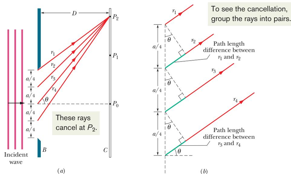
**Fig. 36-6** (a) Waves from the top points of four zones of width  $a/4$  undergo fully destructive interference at point  $P_2$ . (b) For  $D \gg a$ , we can approximate rays  $r_1$ ,  $r_2$ ,  $r_3$ , and  $r_4$  as being parallel, at angle  $\theta$  to the central axis.
