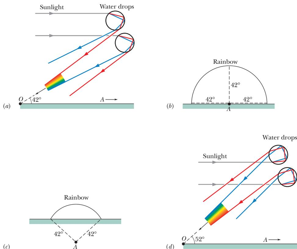
**Fig. 33-21** (a) The separation of colors when sunlight refracts into and out of falling raindrops leads to a primary rainbow. The antisolar point  $A$  is on the horizon at the right. The rainbow colors appear at an angle of  $42^\circ$  from the direction of  $A$ . (b) Drops at  $42^\circ$  from  $A$  in any direction can contribute to the rainbow. (c) The rainbow arc when the Sun is higher (and thus  $A$  is lower). (d) The separation of colors leading to a secondary rainbow.
