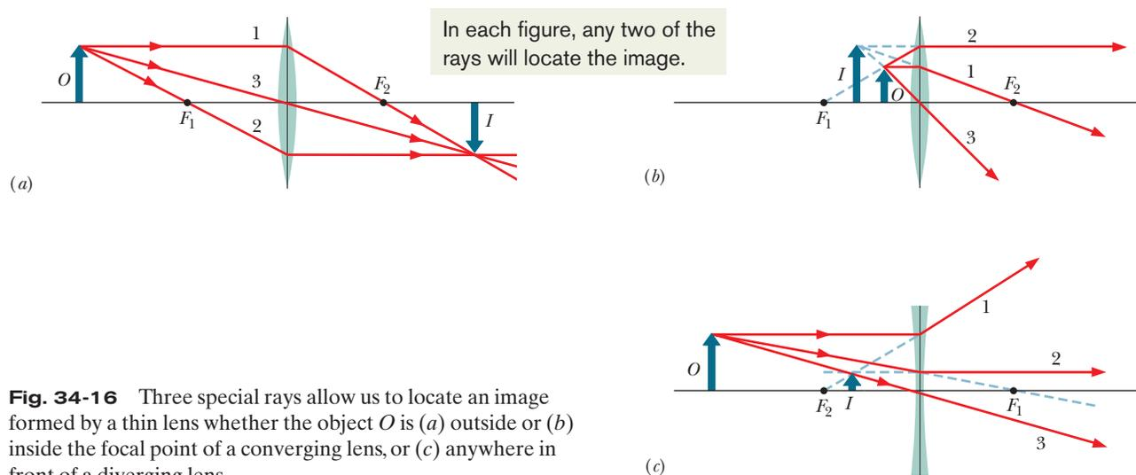
**Fig. 34-16** Three special rays allow us to locate an image formed by a thin lens whether the object  $O$  is (a) outside or (b) inside the focal point of a converging lens, or (c) anywhere in front of a diverging lens.
