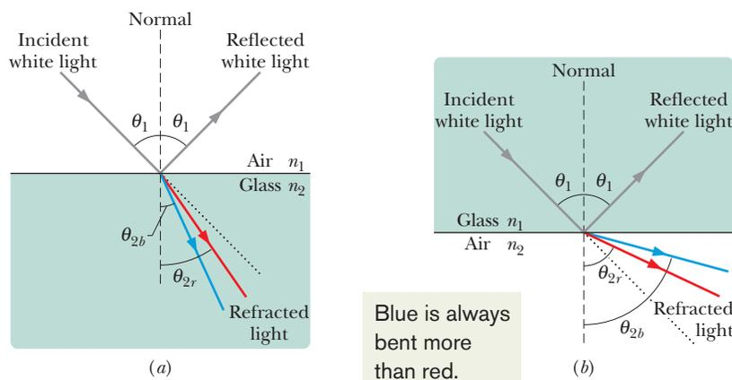
**Fig. 33-19** Chromatic dispersion of white light. The blue component is bent more than the red component. (a) Passing from air to glass, the blue component ends up with the smaller angle of refraction. (b) Passing from glass to air, the blue component ends up with the greater angle of refraction. Each dotted line represents the direction in which the light would continue to travel if it were not bent by the refraction.
