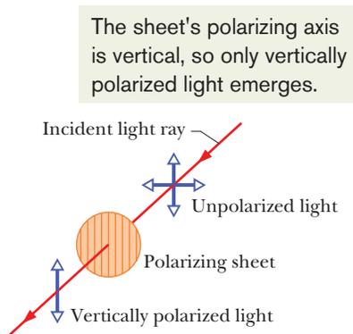
**Fig. 33-11** Unpolarized light becomes polarized when it is sent through a polarizing sheet. Its direction of polarization is then parallel to the polarizing direction of the sheet, which is represented here by the vertical lines drawn in the sheet.
