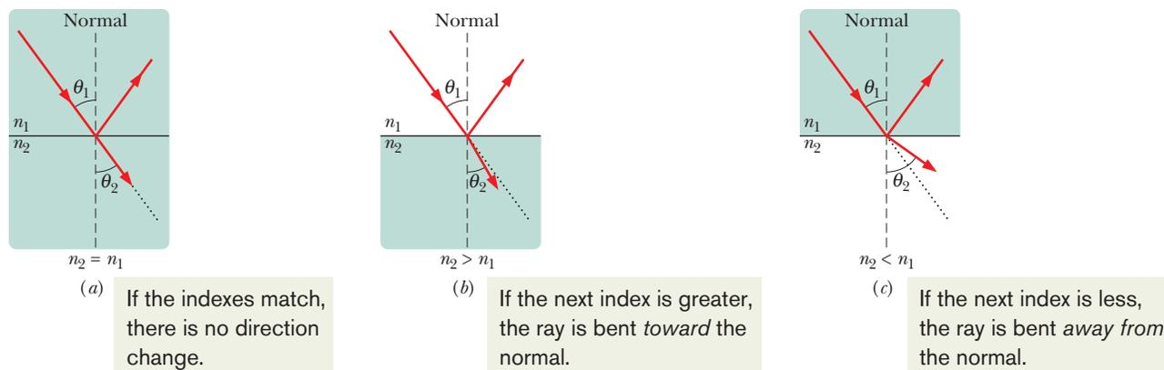
**Fig. 33-17** Refraction of light traveling from a medium with an index of refraction  $n_1$  into a medium with an index of refraction  $n_2$ . (a) The beam does not bend when  $n_2 = n_1$ ; the refracted light then travels in the *undeflected direction* (the dotted line), which is the same as the direction of the incident beam. The beam bends (b) toward the normal when  $n_2 > n_1$  and (c) away from the normal when  $n_2 < n_1$ .
