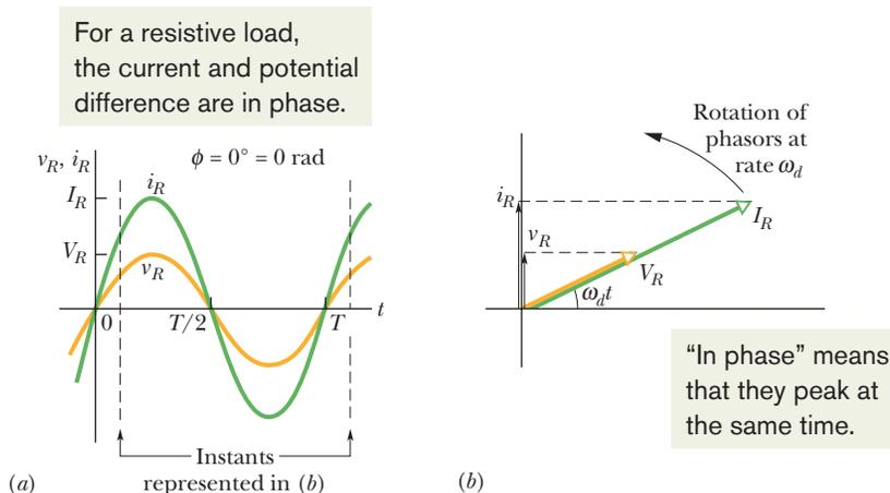
**Fig. 31-9** (a) The current  $i_R$  and the potential difference  $v_R$  across the resistor are plotted on the same graph, both versus time  $t$ . They are in phase and complete one cycle in one period  $T$ . (b) A phasor diagram shows the same thing as (a).
