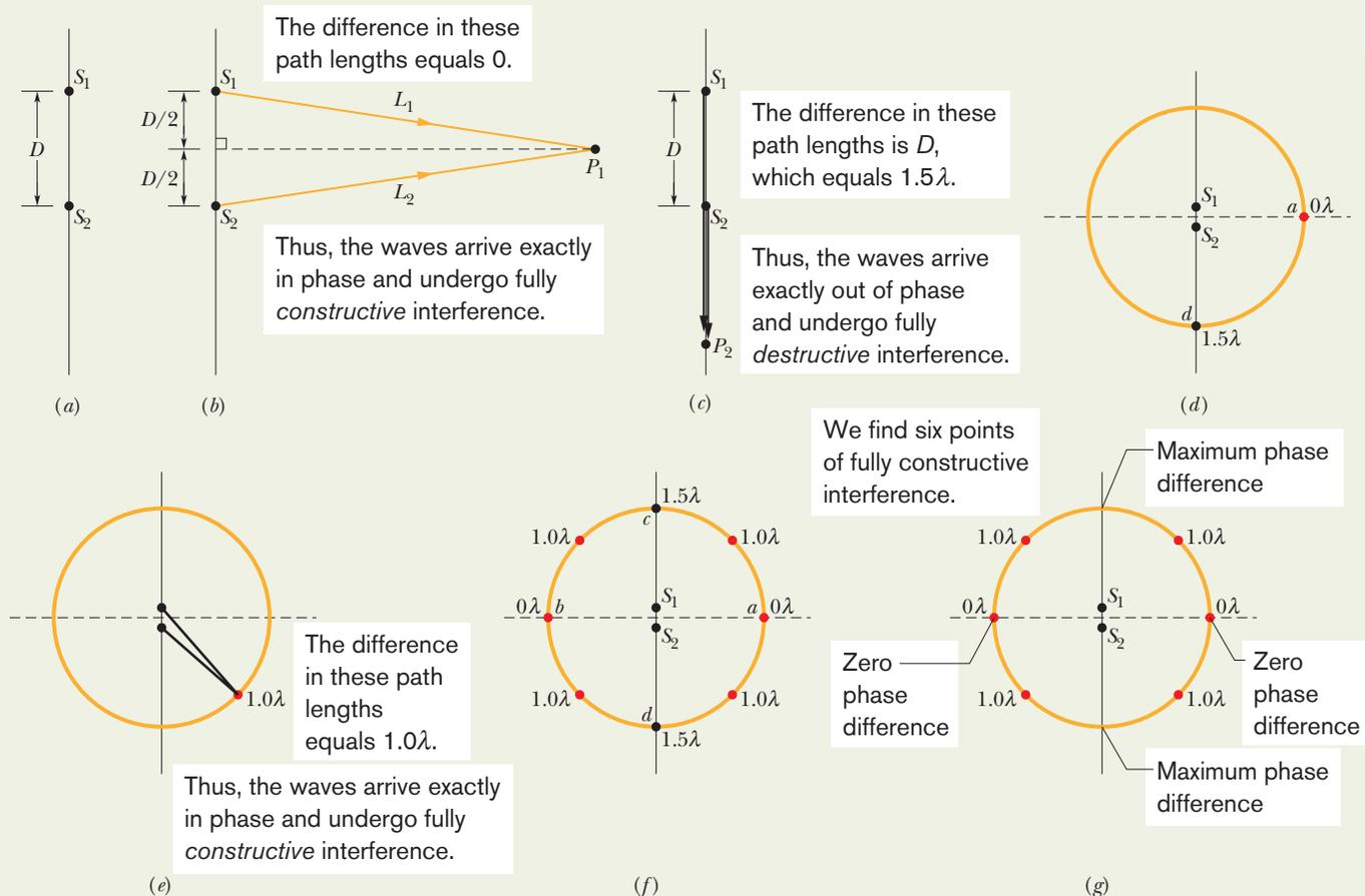
**Fig. 17-8** (a) Two point sources  $S_1$  and  $S_2$ , separated by distance  $D$ , emit spherical sound waves in phase. (b) The waves travel equal distances to reach point  $P_1$ . (c) Point  $P_2$  is on the line extending through  $S_1$  and  $S_2$ . (d) We move around a large circle. (e) Another point of fully constructive interference. (f) Using symmetry to determine other points. (g) The six points of fully constructive interference.
