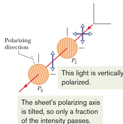
**Fig. 33-13** The light transmitted by polarizing sheet  $P_1$  is vertically polarized, as represented by the vertical double arrow. The amount of that light that is then transmitted by polarizing sheet  $P_2$  depends on the angle between the polarization direction of that light and the polarizing direction of  $P_2$  (indicated by the lines drawn in the sheet and by the dashed line).
