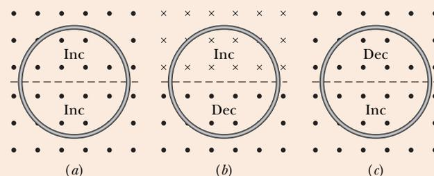
Increasing the external field  $\vec{B}$  induces a current with a field  $\vec{B}_{\text{ind}}$  that opposes the change.
