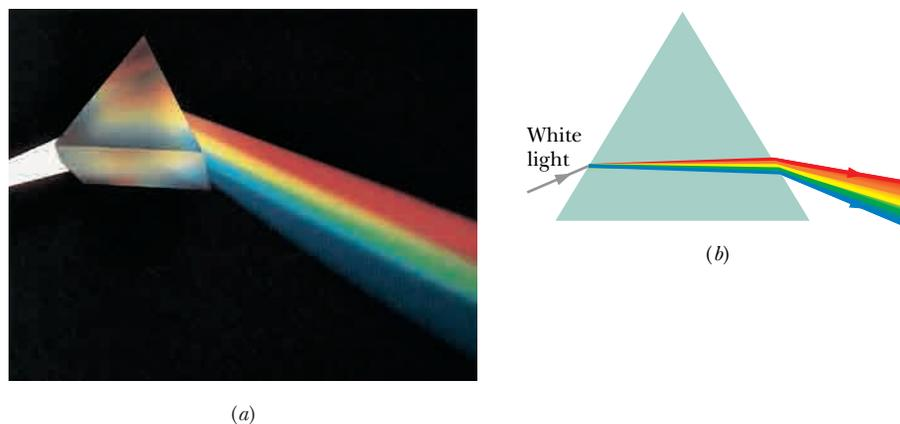
**Fig. 33-20** (a) A triangular prism separating white light into its component colors. (b) Chromatic dispersion occurs at the first surface and is increased at the second surface. (Courtesy Bausch & Lomb)
