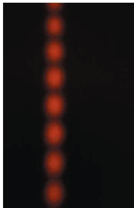
**Fig. 35-9** A photograph of the interference pattern produced by the arrangement shown in Fig. 35-8, but with short slits. (The photograph is a front view of part of screen  $C$ .) The alternating maxima and minima are called *interference fringes* (because they resemble the decorative fringe sometimes used on clothing and rugs). (Jearyl Walker)
