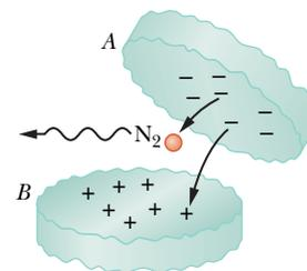
**Fig. 21-5** Two pieces of a wintergreen LifeSaver candy as they fall away from each other. Electrons jumping from the negative surface of piece *A* to the positive surface of piece *B* collide with nitrogen ( $N_2$ ) molecules in the air.
