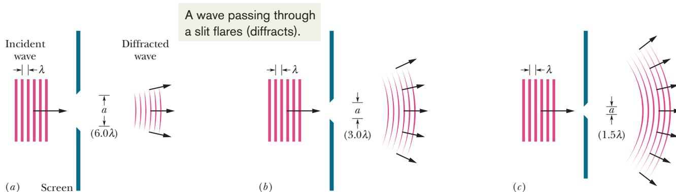
**Fig. 35-7** Diffraction represented schematically. For a given wavelength  $\lambda$ , the diffraction is more pronounced the smaller the slit width  $a$ . The figures show the cases for (a) slit width  $a = 6.0\lambda$ , (b) slit width  $a = 3.0\lambda$ , and (c) slit width  $a = 1.5\lambda$ . In all three cases, the screen and the length of the slit extend well into and out of the page, perpendicular to it.
