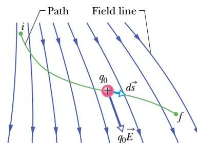
**Fig. 24-4** A test charge  $q_0$  moves from point  $i$  to point  $f$  along the path shown in a nonuniform electric field. During a displacement  $d\vec{s}$ , an electrostatic force  $q_0\vec{E}$  acts on the test charge. This force points in the direction of the field line at the location of the test charge.
