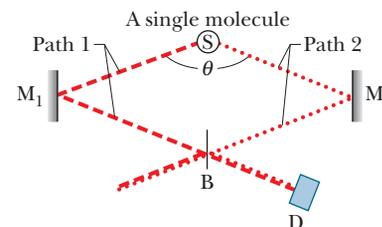
**Fig. 38-7** The light from a single photon emission in source S travels over two widely separated paths and interferes with itself at detector D after being recombined by beam splitter B. (After Ming Lai and Jean-Claude Diels, *Journal of the Optical Society of America B*, **9**, 2290–2294, December 1992.)
