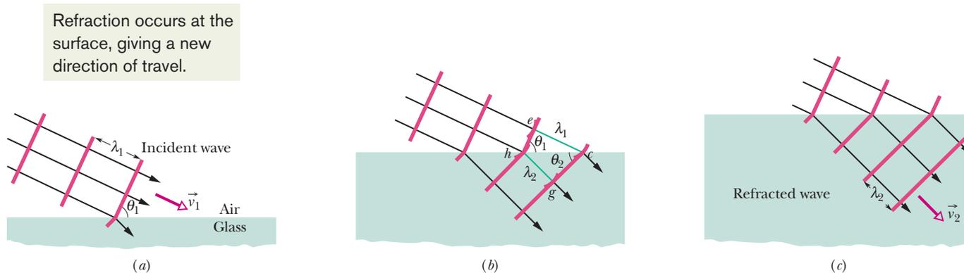
**Fig. 35-3** The refraction of a plane wave at an air–glass interface, as portrayed by Huygens' principle. The wavelength in glass is smaller than that in air. For simplicity, the reflected wave is not shown. Parts (a) through (c) represent three successive stages of the refraction.
