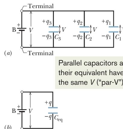
**Fig. 25-8** (a) Three capacitors connected in parallel to battery B. The battery maintains potential difference  $V$  across its terminals and thus across *each* capacitor. (b) The equivalent capacitor, with capacitance  $C_{\text{eq}}$ , replaces the parallel combination.
