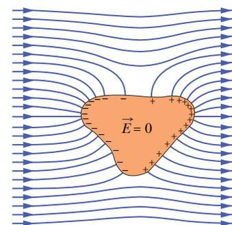
**Fig. 24-20** An uncharged conductor is suspended in an external electric field. The free electrons in the conductor distribute themselves on the surface as shown, so as to reduce the net electric field inside the conductor to zero and make the net field at the surface perpendicular to the surface.
