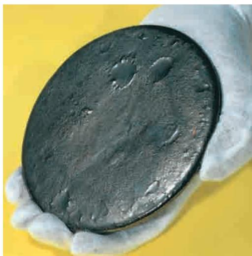
**Fig. 43-14** Problem 15. A “button” of  $^{235}\text{U}$  ready to be recast and machined for a warhead. (*Courtesy Martin Marietta Energy Systems/ U.S. Department of Energy*)
