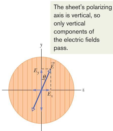
**Fig. 33-12** Polarized light approaching a polarizing sheet. The electric field  $\vec{E}$  of the light can be resolved into components  $E_y$  (parallel to the polarizing direction of the sheet) and  $E_z$  (perpendicular to that direction). Component  $E_y$  will be transmitted by the sheet; component  $E_z$  will be absorbed.
