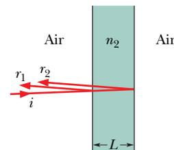
Fig. 35-17 Reflections from a thin film in air.
