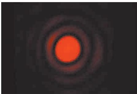
**Fig. 36-10** The diffraction pattern of a circular aperture. Note the central maximum and the circular secondary maxima. The figure has been overexposed to bring out these secondary maxima, which are much less intense than the central maximum. (Jearl Walker)
