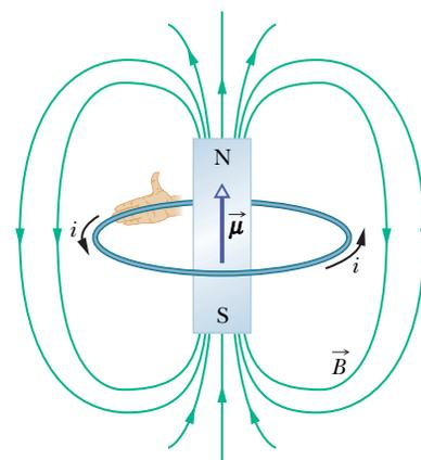
**Fig. 29-21** A current loop produces a magnetic field like that of a bar magnet and thus has associated north and south poles. The magnetic dipole moment  $\vec{\mu}$  of the loop, its direction given by a curled–straight right-hand rule, points from the south pole to the north pole, in the direction of the field  $\vec{B}$  within the loop.
