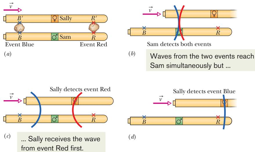
**Fig. 37-4** The spaceships of Sally and Sam and the occurrences of events from Sam's view. Sally's ship moves rightward with velocity  $\vec{v}$ . (a) Event Red occurs at positions  $RR'$  and event Blue occurs at positions  $BB'$ ; each event sends out a wave of light. (b) Sam simultaneously detects the waves from event Red and event Blue. (c) Sally detects the wave from event Red. (d) Sally detects the wave from event Blue.
