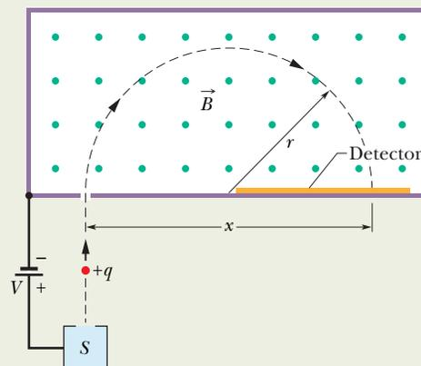
**Fig. 28-12** Essentials of a mass spectrometer. A positive ion, after being accelerated from its source  $S$  by a potential difference  $V$ , enters a chamber of uniform magnetic field  $\vec{B}$ . There it travels through a semicircle of radius  $r$  and strikes a detector at a distance  $x$  from where it entered the chamber.
