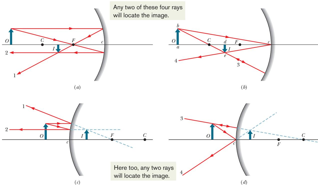
**Fig. 34-11** (a, b) Four rays that may be drawn to find the image formed by a concave mirror. For the object position shown, the image is real, inverted, and smaller than the object. (c, d) Four similar rays for the case of a convex mirror. For a convex mirror, the image is always virtual, oriented like the object, and smaller than the object. [In (c), ray 2 is initially directed toward focal point  $F$ . In (d), ray 3 is initially directed toward center of curvature  $C$ .]
