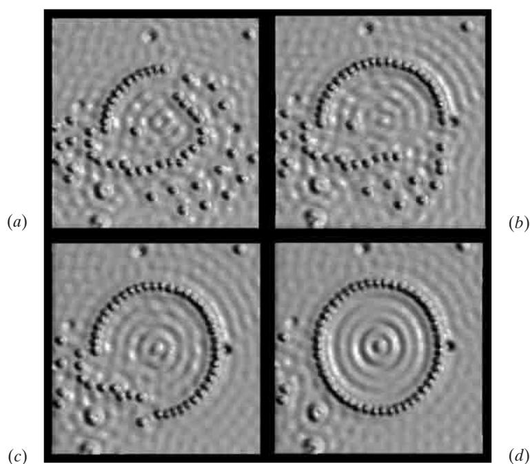
**Fig. 39-12** A quantum corral during four stages of construction. Note the appearance of ripples caused by electrons trapped in the corral when it is almost complete. (Courtesy of International Business Machines Corporation, Almaden Research Center)
