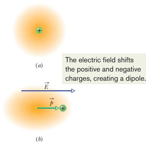
**Fig. 24-11** (a) An atom, showing the positively charged nucleus (green) and the negatively charged electrons (gold shading). The centers of positive and negative charge coincide. (b) If the atom is placed in an external electric field  $\vec{E}$ , the electron orbits are distorted so that the centers of positive and negative charge no longer coincide. An induced dipole moment  $\vec{p}$  appears. The distortion is greatly exaggerated here.
