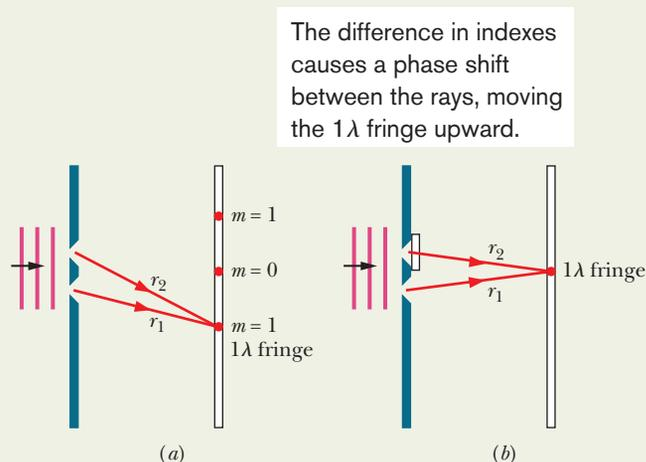
**Fig. 35-11** (a) Arrangement for two-slit interference (not to scale). The locations of three bright fringes (or maxima) are indicated. (b) A strip of plastic covers the top slit. We want the  $1\lambda$  fringe to be at the center of the pattern.
