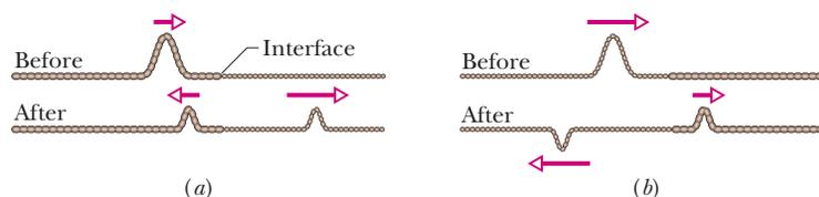
**Fig. 35-16** Phase changes when a pulse is reflected at the interface between two stretched strings of different linear densities. The wave speed is greater in the lighter string. (a) The incident pulse is in the denser string. (b) The incident pulse is in the lighter string. Only here is there a phase change, and only in the reflected wave.
