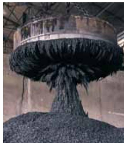
**Fig. 28-1** Using an electromagnet to collect and transport scrap metal at a steel mill. (Digital Vision/Getty Images)
