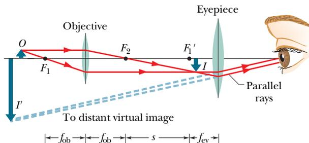
**Fig. 34-20** A thin-lens representation of a compound microscope (not to scale). The objective produces a real image  $I$  of object  $O$  just inside the focal point  $F_1'$  of the eyepiece. Image  $I$  then acts as an object for the eyepiece, which produces a virtual final image  $I'$  that is seen by the observer. The objective has focal length  $f_{ob}$ ; the eyepiece has focal length  $f_{ey}$ ; and  $s$  is the tube length.
