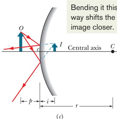
**Fig. 34-8** (a) An object  $O$  forms a virtual image  $I$  in a plane mirror. (b) If the mirror is bent so that it becomes *concave*, the image moves farther away and becomes larger. (c) If the plane mirror is bent so that it becomes *convex*, the image moves closer and becomes smaller.
