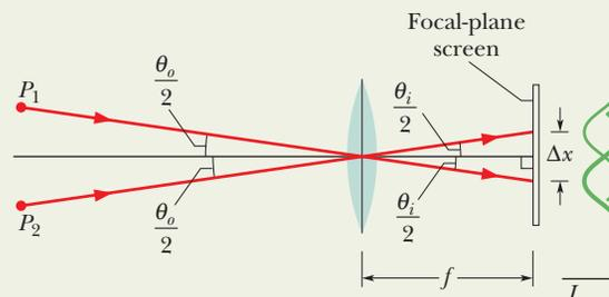
**Fig. 36-14** Light from two distant point objects  $P_1$  and  $P_2$  passes through a converging lens and forms images on a viewing screen in the focal plane of the lens. Only one representative ray from each object is shown. The images are not points but diffraction patterns, with intensities approximately as plotted at the right. The angular separation of the objects is  $\theta_o$  and that of the images is  $\theta_i$ ; the central maxima of the images have a separation  $\Delta x$ .
