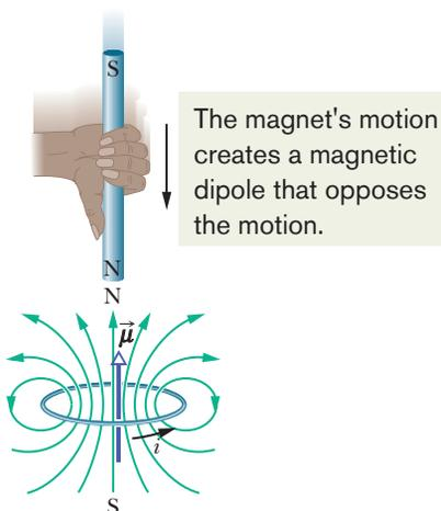
**Fig. 30-4** Lenz's law at work. As the magnet is moved toward the loop, a current is induced in the loop. The current produces its own magnetic field, with magnetic dipole moment  $\vec{\mu}$  oriented so as to oppose the motion of the magnet. Thus, the induced current must be counterclockwise as shown.
