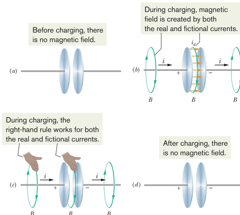
**Fig. 32-7** (a) Before and (d) after the plates are charged, there is no magnetic field. (b) During the charging, magnetic field is created by both the real current and the (fictional) displacement current. (c) The same right-hand rule works for both currents to give the direction of the magnetic field.
