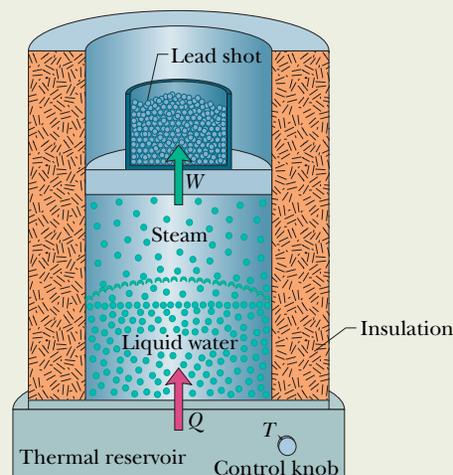
**Fig. 18-17** Water boiling at constant pressure. Energy is transferred from the thermal reservoir as heat until the liquid water has changed completely into steam. Work is done by the expanding gas as it lifts the loaded piston.
