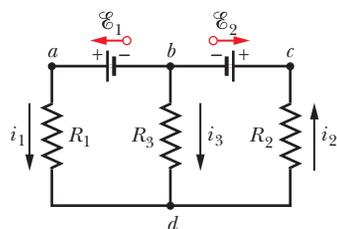
**Fig. 27-9** A multiloop circuit consisting of three branches: left-hand branch  $bad$ , right-hand branch  $bcd$ , and central branch  $bd$ . The circuit also consists of three loops: left-hand loop  $badb$ , right-hand loop  $bcd b$ , and big loop  $badcb$ .
