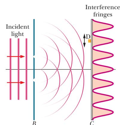
**Fig. 38-6** Light is directed onto screen  $B$ , which contains two parallel slits. Light emerging from these slits spreads out by diffraction. The two diffracted waves overlap at screen  $C$  and form a pattern of interference fringes. A small photon detector  $D$  in the plane of screen  $C$  generates a sharp click for each photon that it absorbs.
