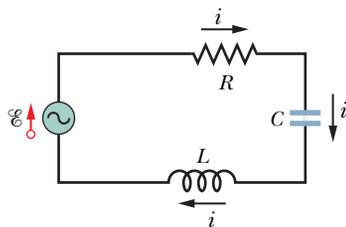
**Fig. 31-7** A single-loop circuit containing a resistor, a capacitor, and an inductor. A generator, represented by a sine wave in a circle, produces an alternating emf that establishes an alternating current; the directions of the emf and current are indicated here at only one instant.
