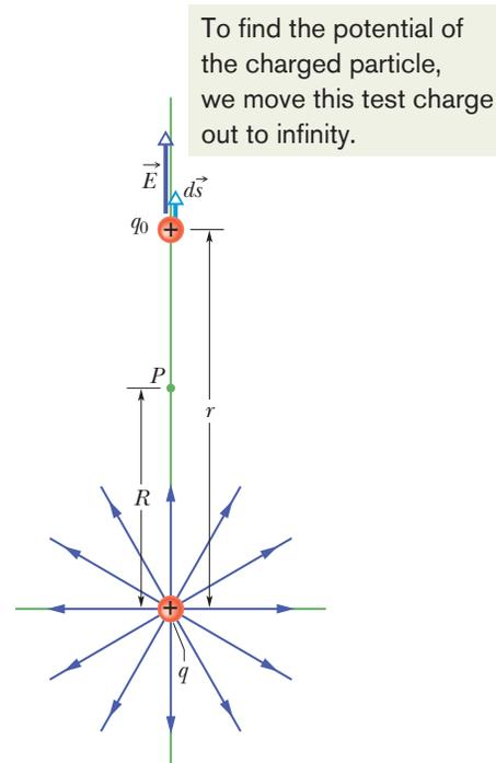
**Fig. 24-6** The positive point charge  $q$  produces an electric field  $\vec{E}$  and an electric potential  $V$  at point  $P$ . We find the potential by moving a test charge  $q_0$  from  $P$  to infinity. The test charge is shown at distance  $r$  from the point charge, during differential displacement  $d\vec{s}$ .
