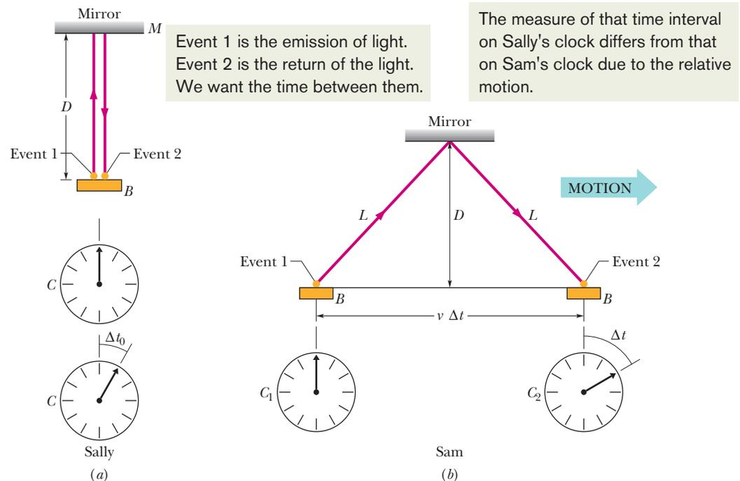
**Fig. 37-5** (a) Sally, on the train, measures the time interval  $\Delta t_0$  between events 1 and 2 using a single clock  $C$  on the train. That clock is shown twice: first for event 1 and then for event 2. (b) Sam, watching from the station as the events occur, requires two synchronized clocks,  $C_1$  at event 1 and  $C_2$  at event 2, to measure the time interval between the two events; his measured time interval is  $\Delta t$ .
