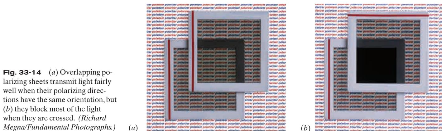
**Fig. 33-14** (a) Overlapping polarizing sheets transmit light fairly well when their polarizing directions have the same orientation, but (b) they block most of the light when they are crossed. (Richard Megna/Fundamental Photographs.)
