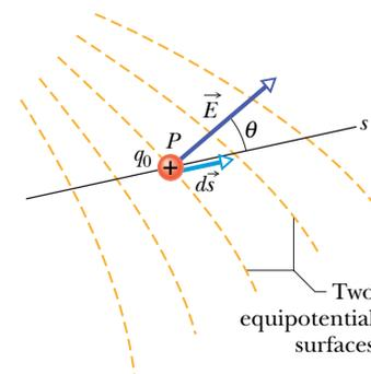
**Fig. 24-14** A test charge  $q_0$  moves a distance  $d\vec{s}$  from one equipotential surface to another. (The separation between the surfaces has been exaggerated for clarity.) The displacement  $d\vec{s}$  makes an angle  $\theta$  with the direction of the electric field  $\vec{E}$ .
