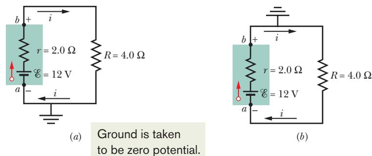
**Fig. 27-7** (a) Point  $a$  is directly connected to ground. (b) Point  $b$  is directly connected to ground.
