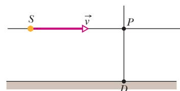
**Fig. 37-12** A light source  $S$  travels with velocity  $\vec{v}$  past a detector at  $D$ . The special theory of relativity predicts a transverse Doppler effect as the source passes through point  $P$ , where the direction of travel is perpendicular to the line extending through  $D$ . Classical theory predicts no such effect.
