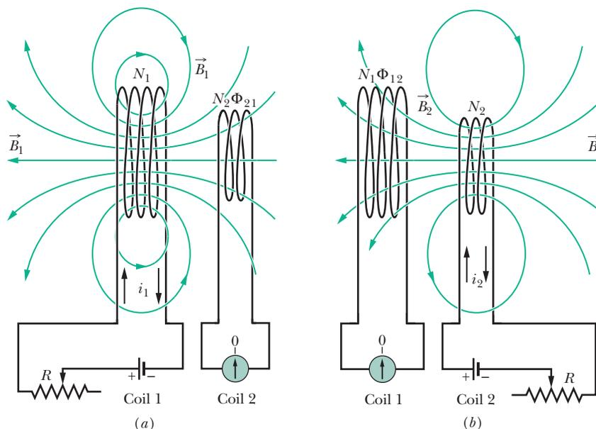
**Fig. 30-19** Mutual induction. (a) The magnetic field  $\vec{B}_1$  produced by current  $i_1$  in coil 1 extends through coil 2. If  $i_1$  is varied (by varying resistance  $R$ ), an emf is induced in coil 2 and current registers on the meter connected to coil 2. (b) The roles of the coils interchanged.
