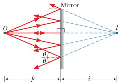
**Fig. 34-2** A point source of light  $O$ , called the *object*, is a perpendicular distance  $p$  in front of a plane mirror. Light rays reaching the mirror from  $O$  reflect from the mirror. If your eye intercepts some of the reflected rays, you perceive a point source of light  $I$  to be behind the mirror, at a perpendicular distance  $i$ . The perceived source  $I$  is a virtual image of object  $O$ .
