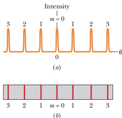
**Fig. 36-19** (a) The intensity plot produced by a diffraction grating with a great many rulings consists of narrow peaks, here labeled with their order numbers  $m$ . (b) The corresponding bright fringes seen on the screen are called lines and are here also labeled with order numbers  $m$ .
