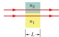
**Fig. 35-4** Two light rays travel through two media having different indexes of refraction.
