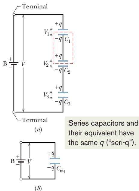
**Fig. 25-9** (a) Three capacitors connected in series to battery B. The battery maintains potential difference  $V$  between the top and bottom plates of the series combination. (b) The equivalent capacitor, with capacitance  $C_{\text{eq}}$ , replaces the series combination.
