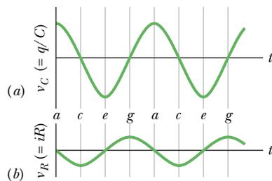
**Fig. 31-2** (a) The potential difference across the capacitor of the circuit of Fig. 31-1 as a function of time. This quantity is proportional to the charge on the capacitor. (b) A potential proportional to the current in the circuit of Fig. 31-1. The letters refer to the correspondingly labeled oscillation stages in Fig. 31-1.
