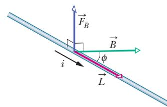
**Fig. 28-16** A wire carrying current  $i$  makes an angle  $\phi$  with magnetic field  $\vec{B}$ . The wire has length  $L$  in the field and length vector  $\vec{L}$  (in the direction of the current). A magnetic force  $\vec{F}_B = i\vec{L} \times \vec{B}$  acts on the wire.
