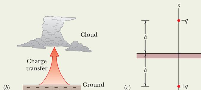
**Fig. 22-9** (a) Photograph of a sprite. (Courtesy NASA) (b) Lightning in which a large amount of negative charge is transferred from ground to cloud base. (c) The cloud-ground system modeled as a vertical electric dipole.
