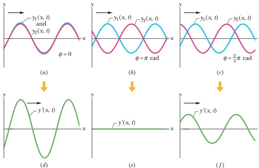
**Fig. 16-13** Two identical sinusoidal waves,  $y_1(x,t)$  and  $y_2(x,t)$ , travel along a string in the positive direction of an  $x$  axis. They interfere to give a resultant wave  $y'(x,t)$ . The resultant wave is what is actually seen on the string. The phase difference  $\phi$  between the two interfering waves is (a) 0 rad or  $0^\circ$ , (b)  $\pi$  rad or  $180^\circ$ , and (c)  $\frac{2}{3}\pi$  rad or  $120^\circ$ . The corresponding resultant waves are shown in (d), (e), and (f).
