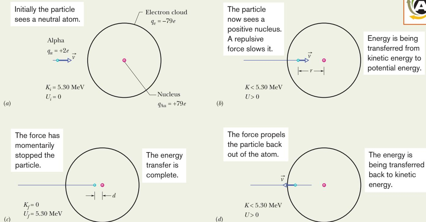
**Fig. 42-4** An alpha particle (a) approaches and (b) then enters a gold atom, headed toward the nucleus. The alpha particle (c) comes to a stop at the point of closest approach and (d) is propelled back out of the atom.
