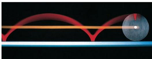
**Fig. 11-2** A time-exposure photograph of a rolling disk. Small lights have been attached to the disk, one at its center and one at its edge. The latter traces out a curve called a *cycloid*. (Richard Megna/Fundamental Photographs)
