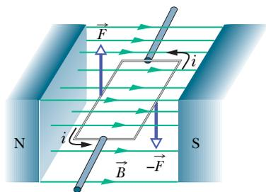
**Fig. 28-18** The elements of an electric motor. A rectangular loop of wire, carrying a current and free to rotate about a fixed axis, is placed in a magnetic field. Magnetic forces on the wire produce a torque that rotates it. A commutator (not shown) reverses the direction of the current every half-revolution so that the torque always acts in the same direction.
