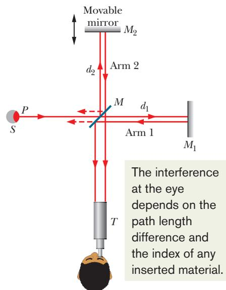
**Fig. 35-21** Michelson's interferometer, showing the path of light originating at point  $P$  of an extended source  $S$ . Mirror  $M$  splits the light into two beams, which reflect from mirrors  $M_1$  and  $M_2$  back to  $M$  and then to telescope  $T$ . In the telescope an observer sees a pattern of interference fringes.
