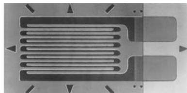
**Fig. 12-13** A strain gage of overall dimensions 9.8 mm by 4.6 mm. The gage is fastened with adhesive to the object whose strain is to be measured; it experiences the same strain as the object. The electrical resistance of the gage varies with the strain, permitting strains up to 3% to be measured. (Courtesy Vishay Micro-Measurements Group, Raleigh, NC)
