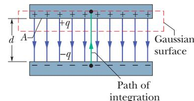
**Fig. 25-5** A charged parallel-plate capacitor. A Gaussian surface encloses the charge on the positive plate. The integration of Eq. 25-6 is taken along a path extending directly from the negative plate to the positive plate.
