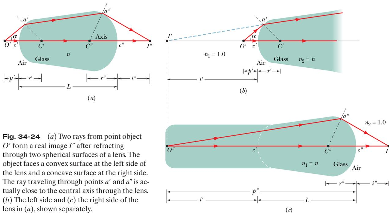
**Fig. 34-24** (a) Two rays from point object  $O'$  form a real image  $I''$  after refracting through two spherical surfaces of a lens. The object faces a convex surface at the left side of the lens and a concave surface at the right side. The ray traveling through points  $a'$  and  $a''$  is actually close to the central axis through the lens. (b) The left side and (c) the right side of the lens in (a), shown separately.
