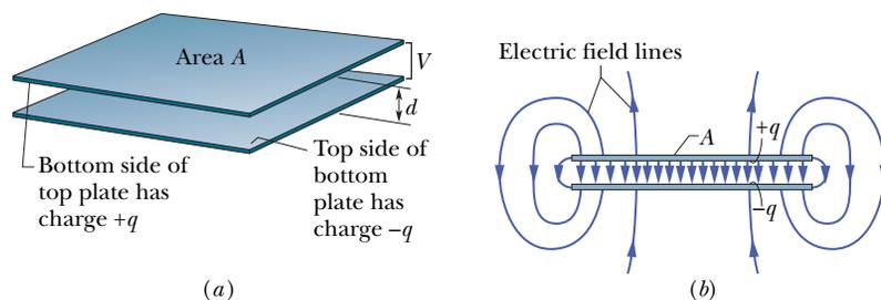
**Fig. 25-3** (a) A parallel-plate capacitor, made up of two plates of area  $A$  separated by a distance  $d$ . The charges on the facing plate surfaces have the same magnitude  $q$  but opposite signs. (b) As the field lines show, the electric field due to the charged plates is uniform in the central region between the plates. The field is not uniform at the edges of the plates, as indicated by the “fringing” of the field lines there.
