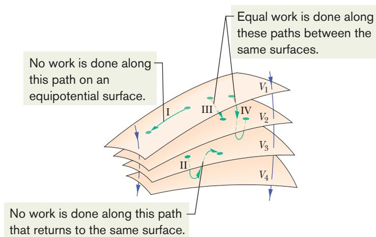
**Fig. 24-2** Portions of four equipotential surfaces at electric potentials  $V_1 = 100$  V,  $V_2 = 80$  V,  $V_3 = 60$  V, and  $V_4 = 40$  V. Four paths along which a test charge may move are shown. Two electric field lines are also indicated.
