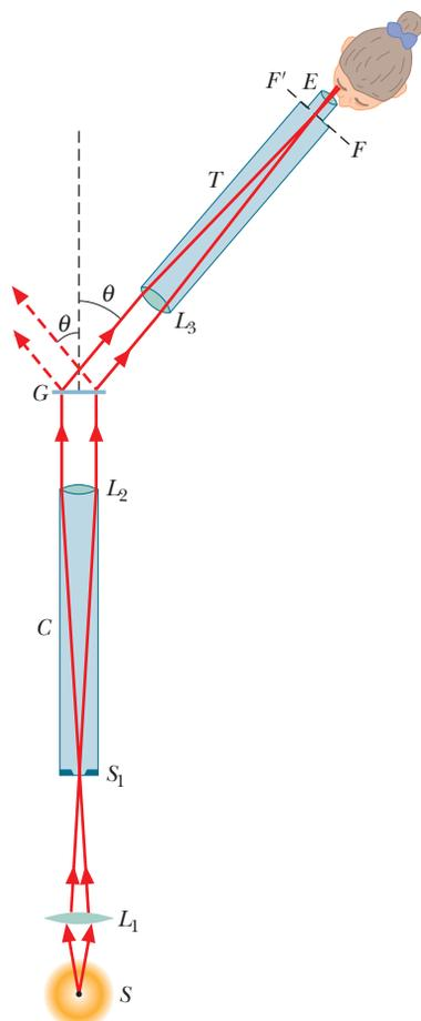
**Fig. 36-23** A simple type of grating spectroscope used to analyze the wavelengths of light emitted by source  $S$ .
