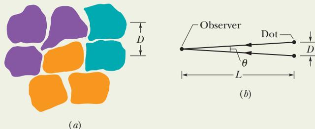
**Fig. 36-13** (a) Representation of some dots on a pointillistic painting, showing an average center-to-center separation  $D$ . (b) The arrangement of separation  $D$  between two dots, their angular separation  $\theta$ , and the viewing distance  $L$ .
