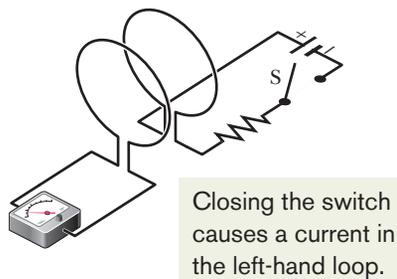
**Fig. 30-2** An ammeter registers a current in the left-hand wire loop just as switch S is closed (to turn on the current in the right-hand wire loop) or opened (to turn off the current in the right-hand loop). No motion of the coils is involved.
