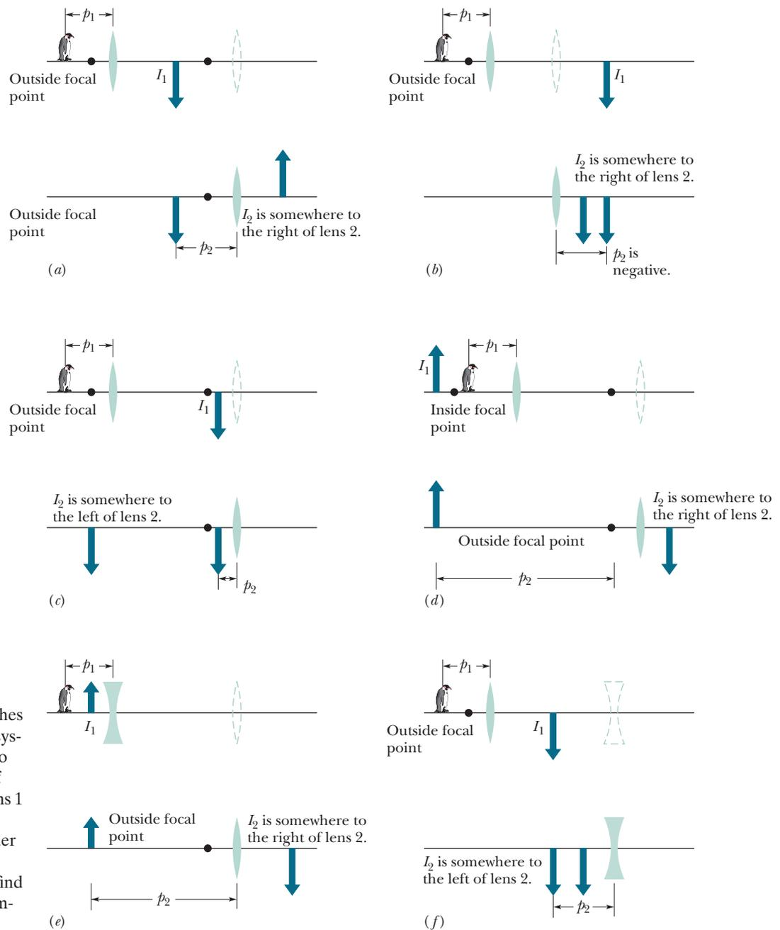
**Fig. 34-17** Several sketches (not to scale) of a two-lens system in which an object sits to the left of lens 1. In step 1 of the solution, we consider lens 1 and ignore lens 2 (shown in dashes). In step 2, we consider lens 2 and ignore lens 1 (no longer shown). We want to find the final image, that is, the image produced by lens 2.
