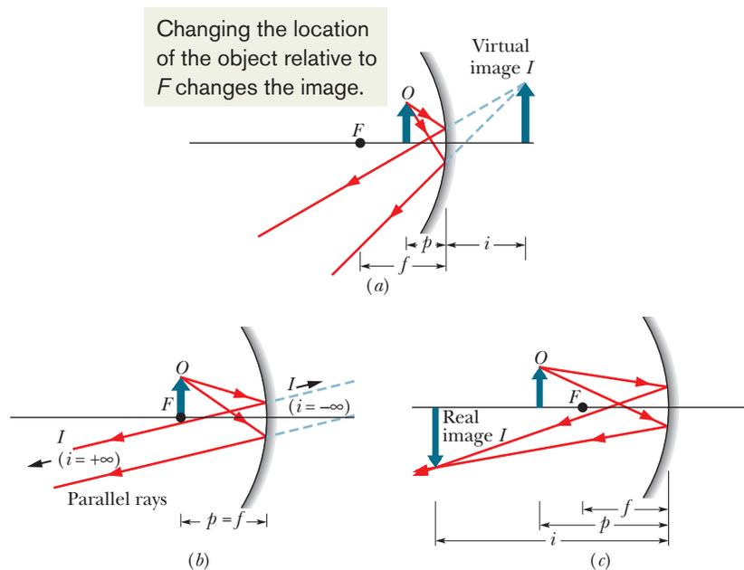
**Fig. 34-10** (a) An object  $O$  inside the focal point of a concave mirror, and its virtual image  $I$ . (b) The object at the focal point  $F$ . (c) The object outside the focal point, and its real image  $I$ .
