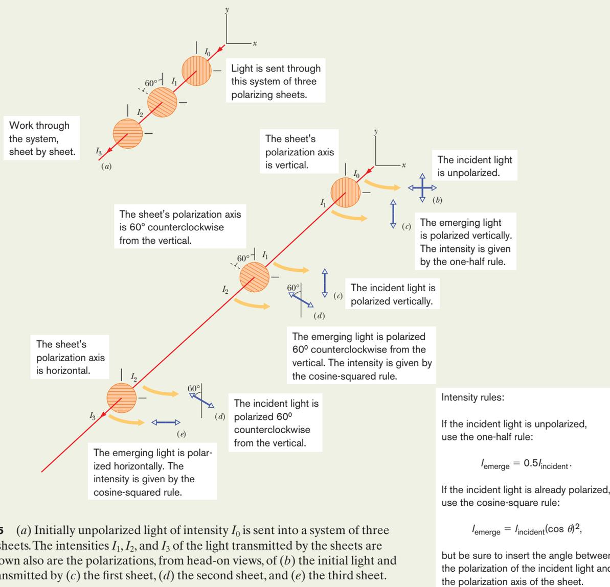
**Fig. 33-15** (a) Initially unpolarized light of intensity  $I_0$  is sent into a system of three polarizing sheets. The intensities  $I_1$ ,  $I_2$ , and  $I_3$  of the light transmitted by the sheets are labeled. Shown also are the polarizations, from head-on views, of (b) the initial light and the light transmitted by (c) the first sheet, (d) the second sheet, and (e) the third sheet.
