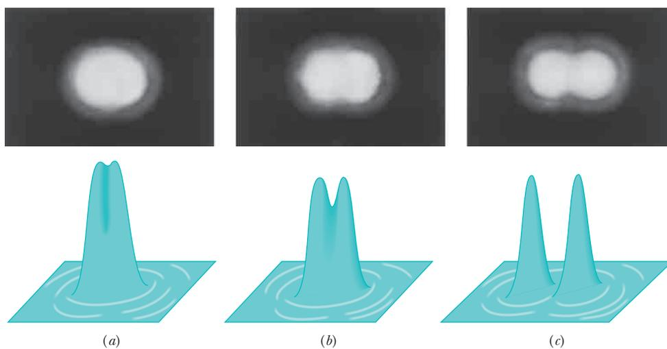
**Fig. 36-11** At the top, the images of two point sources (stars) formed by a converging lens. At the bottom, representations of the image intensities. In (a) the angular separation of the sources is too small for them to be distinguished, in (b) they can be marginally distinguished, and in (c) they are clearly distinguished. Rayleigh's criterion is satisfied in (b), with the central maximum of one diffraction pattern coinciding with the first minimum of the other.
