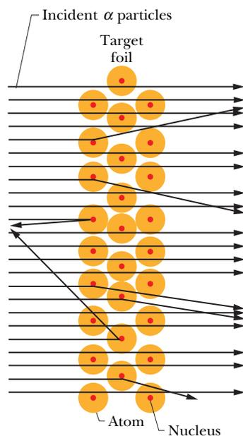
**Fig. 42-3** The angle through which an incident alpha particle is scattered depends on how close the particle's path lies to an atomic nucleus. Large deflections result only from very close encounters.
