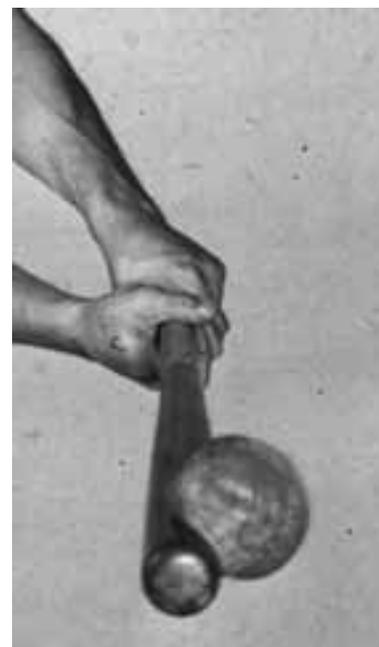
The collision of a ball with a bat collapses part of the ball. (Photo by Harold E. Edgerton. ©The Harold and Esther Edgerton Family Trust, courtesy of Palm Press, Inc.)
