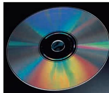
The fine rulings, each  $0.5 \mu\text{m}$  wide, on a compact disc function as a diffraction grating. When a small source of white light illuminates a disc, the diffracted light forms colored “lanes” that are the composite of the diffraction patterns from the rulings.
