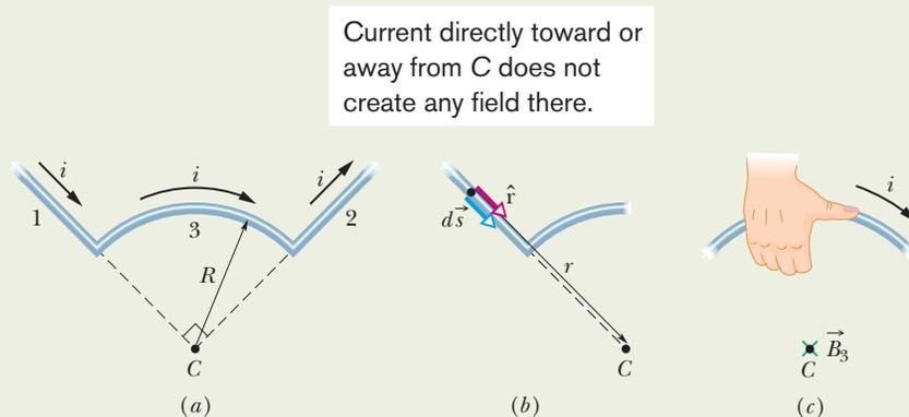
**Fig. 29-7** (a) A wire consists of two straight sections (1 and 2) and a circular arc (3), and carries current  $i$ . (b) For a current-length element in section 1, the angle between  $d\vec{s}$  and  $\hat{r}$  is zero. (c) Determining the direction of magnetic field  $\vec{B}_3$  at  $C$  due to the current in the circular arc; the field is into the page there.
