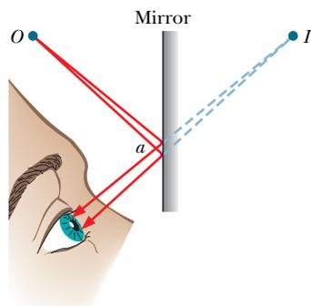
**Fig. 34-4** A “pencil” of rays from  $O$  enters the eye after reflection at the mirror. Only a small portion of the mirror near  $a$  is involved in this reflection. The light appears to originate at point  $I$  behind the mirror.
