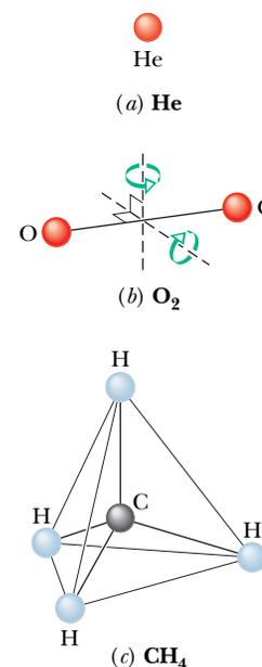
**Fig. 19-13** Models of molecules as used in kinetic theory: (a) helium, a typical monatomic molecule; (b) oxygen, a typical diatomic molecule; and (c) methane, a typical polyatomic molecule. The spheres represent atoms, and the lines between them represent bonds. Two rotation axes are shown for the oxygen molecule.
