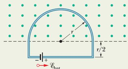
**Fig. 30-6** A battery is connected to a conducting loop that includes a half-circle of radius  $r$  lying in a uniform magnetic field. The field is directed out of the page; its magnitude is changing.
