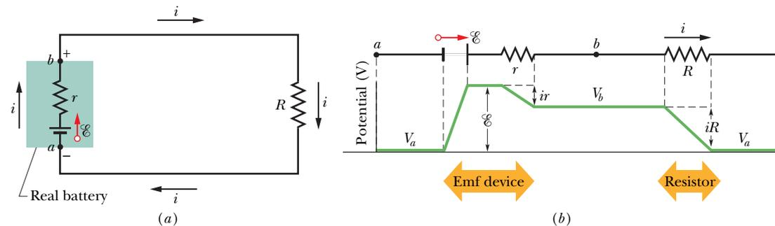
**Fig. 27-4** (a) A single-loop circuit containing a real battery having internal resistance  $r$  and emf  $\mathcal{E}$ . (b) The same circuit, now spread out in a line. The potentials encountered in traversing the circuit clockwise from  $a$  are also shown. The potential  $V_a$  is arbitrarily assigned a value of zero, and other potentials in the circuit are graphed relative to  $V_a$ .
