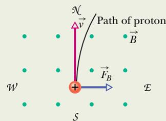
**Fig. 28-6** An overhead view of a proton moving from south to north with velocity  $\vec{v}$  in a chamber. A magnetic field is directed vertically upward in the chamber, as represented by the array of dots (which resemble the tips of arrows). The proton is deflected toward the east.
