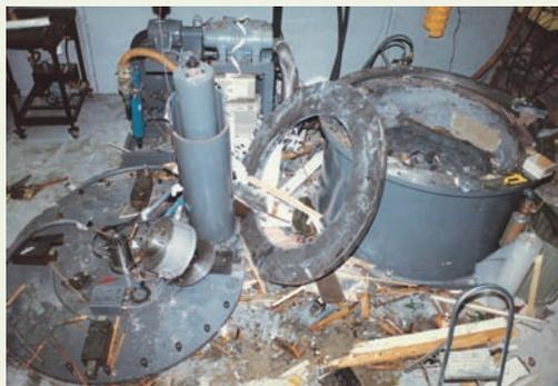
Fig. 10-15 Some of the destruction caused by the explosion of a rapidly rotating steel disk. (Courtesy Test Devices, Inc.)
