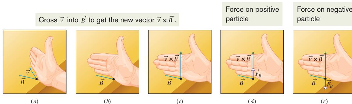
**Fig. 28-2** (a)–(c) The right-hand rule (in which  $\vec{v}$  is swept into  $\vec{B}$  through the smaller angle  $\phi$  between them) gives the direction of  $\vec{v} \times \vec{B}$  as the direction of the thumb. (d) If  $q$  is positive, then the direction of  $\vec{F}_B = q\vec{v} \times \vec{B}$  is in the direction of  $\vec{v} \times \vec{B}$ . (e) If  $q$  is negative, then the direction of  $\vec{F}_B$  is opposite that of  $\vec{v} \times \vec{B}$ .
