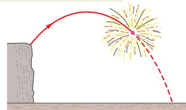
**Fig. 9-5** A fireworks rocket explodes in flight. In the absence of air drag, the center of mass of the fragments would continue to follow the original parabolic path, until fragments began to hit the ground.
