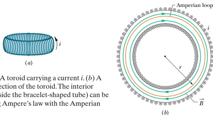
**Fig. 29-20** (a) A toroid carrying a current  $i$ . (b) A horizontal cross section of the toroid. The interior magnetic field (inside the bracelet-shaped tube) can be found by applying Ampere's law with the Amperian loop shown.
