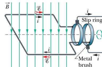
**Fig. 31-6** The basic mechanism of an alternating-current generator is a conducting loop rotated in an external magnetic field. In practice, the alternating emf induced in a coil of many turns of wire is made accessible by means of slip rings attached to the rotating loop. Each ring is connected to one end of the loop wire and is electrically connected to the rest of the generator circuit by a conducting brush against which the ring slips as the loop (and it) rotates.
