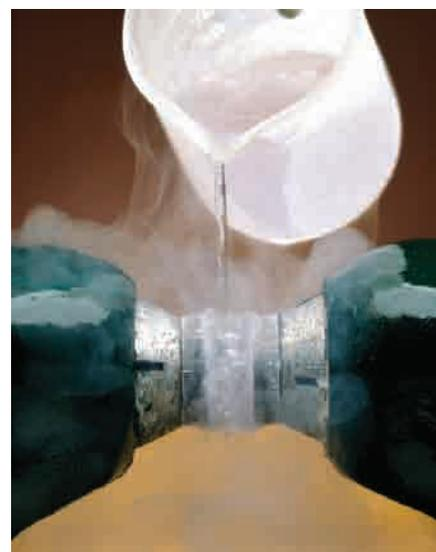
Liquid oxygen is suspended between the two pole faces of a magnet because the liquid is paramagnetic and is magnetically attracted to the magnet. (Richard Megna/Fundamental Photographs)
