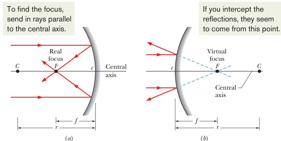
**Fig. 34-9** (a) In a concave mirror, incident parallel light rays are brought to a real focus at  $F$ , on the same side of the mirror as the incident light rays. (b) In a convex mirror, incident parallel light rays seem to diverge from a virtual focus at  $F$ , on the side of the mirror opposite the light rays.
