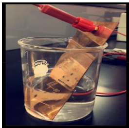
Figure 8 : Copper and carbon cathodes
