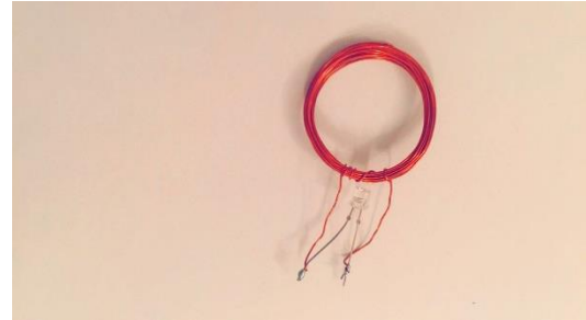
Figure (3.3) power receiver
