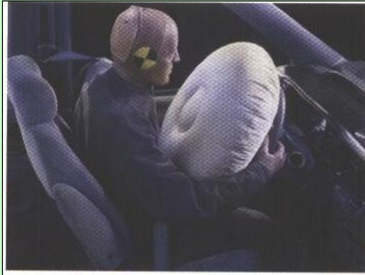
Fig. 55 : Automobile air bags are inflated with \text{N}_2 gas produced by decomposition of sodium azide
