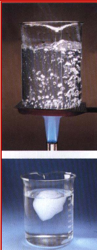
Fig. 50 : During any phase change, liquid \rightleftharpoons gas and solid \rightleftharpoons liquid the temperature remains constant.
