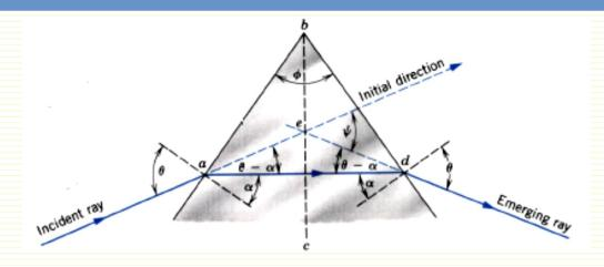
Note that  $\angle bad + \alpha = \pi/2$  and that  $\angle bad + \phi/2 = \pi/2$ , where  $\phi$  is the prism angle. Therefore
