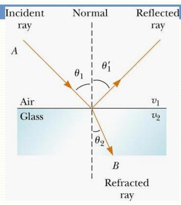
$$n = \frac{c}{v} = \frac{speed\ of\ light\ in\ vacuum}{speed\ of\ light\ in\ medium}$$
