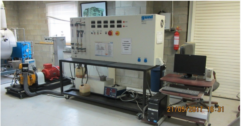
Figure 13.10. Single cylinder variable compression-ratio petrol engine (full computerized and monitored), with extended exhaust gases flexible tubular manifold through the main out-door exit.
