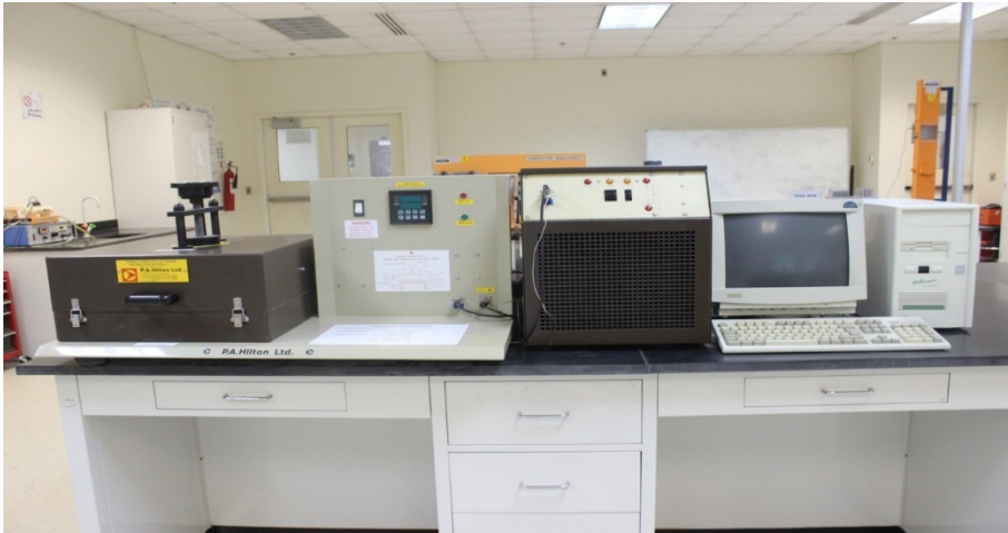
Figure 11.8 Measurement of building materials thermal conductivity unit
