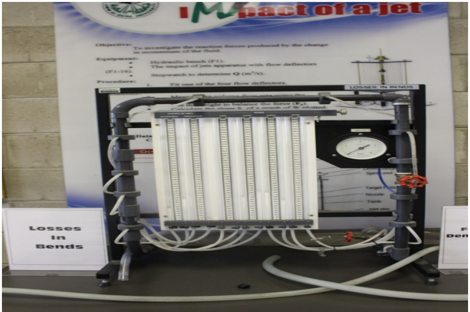
Figure 12.6 Test-rig of measuring the pressure loss in bends & valves.
