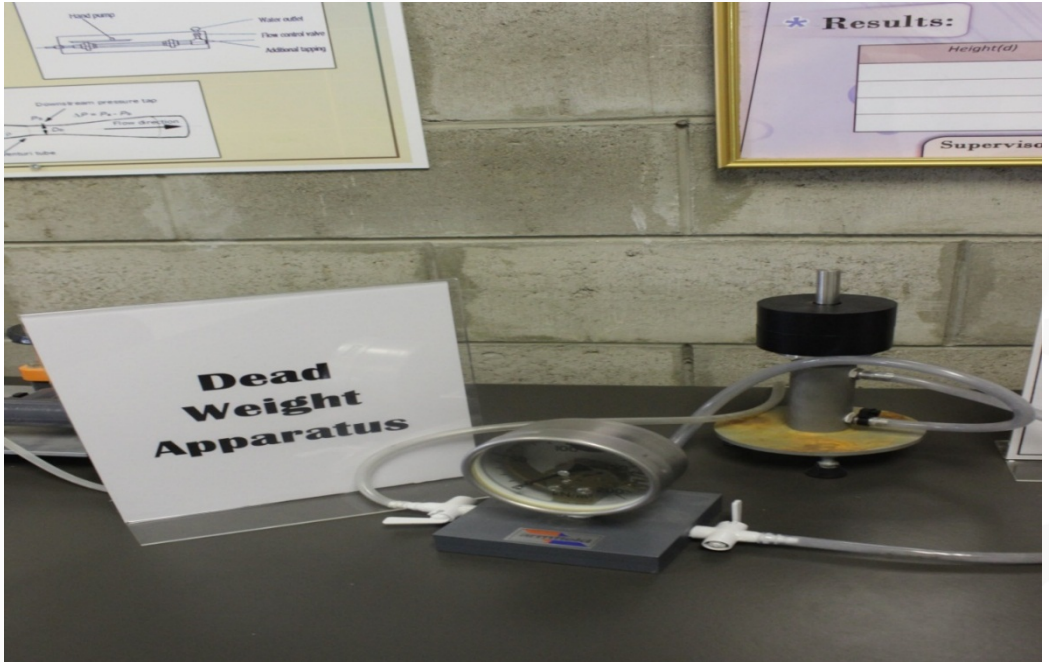
Figure 12.3 Dead weight apparatus (used for manometers calibration).
