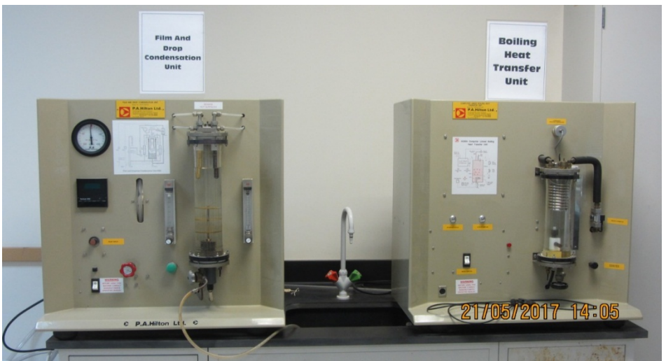
Figure 11.7 (a) Film & drops condensation heat transfer unit (forced water circulation is missed, stopped running) (b) Boiling heat transfer unit
