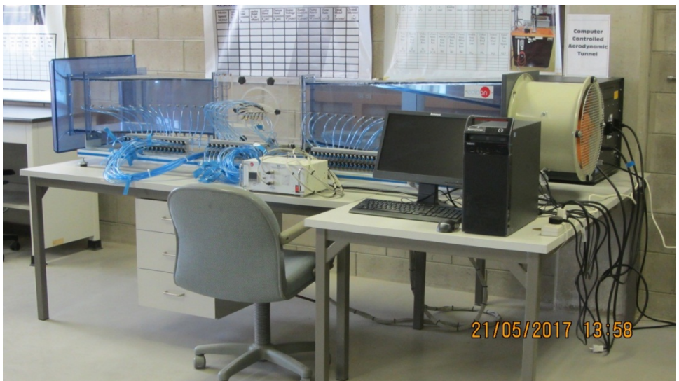
Figure 12.9 Computerized controlled aerodynamics wind tunnel study unit.
