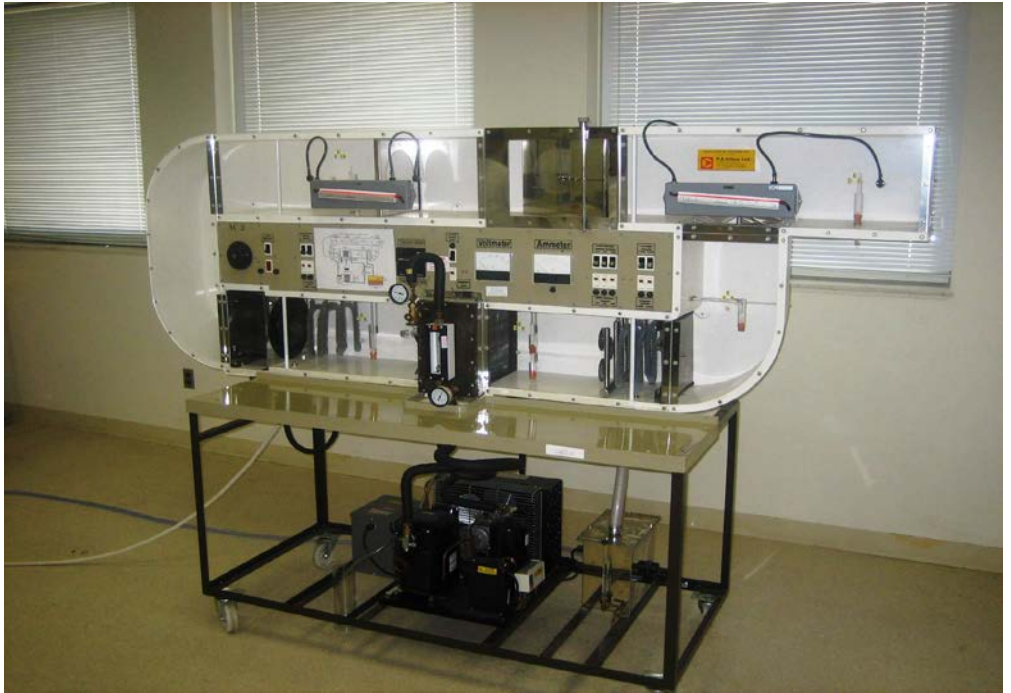
Figure 10.4 Industrial training recirculating air-Conditioning unit.
