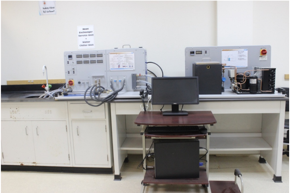
Figure 11.6 Experimental "water heat-exchanger" effectiveness study unit, including "refrigeration unit" for controlled cooling-water system.
