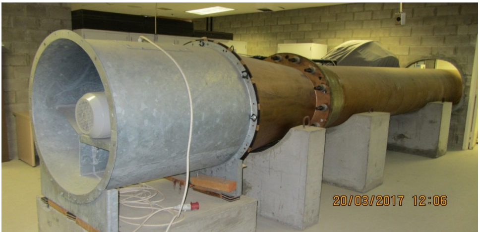
Figure 13.8 Motor side of a wind tunnel occupying about half of the graduate project zone (left- side).
