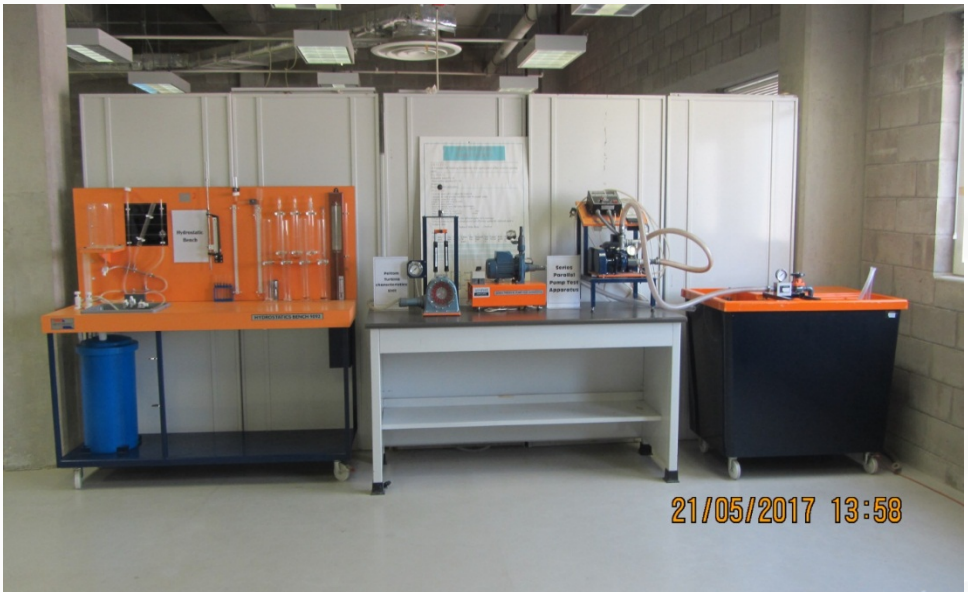
Figure 12.8 (a) Series & parallel water pumps test-rig (right-hand), (b) Pelton water turbine characteristics test-rig (middle), and (c) Hydrostatic bench (left-hand).
