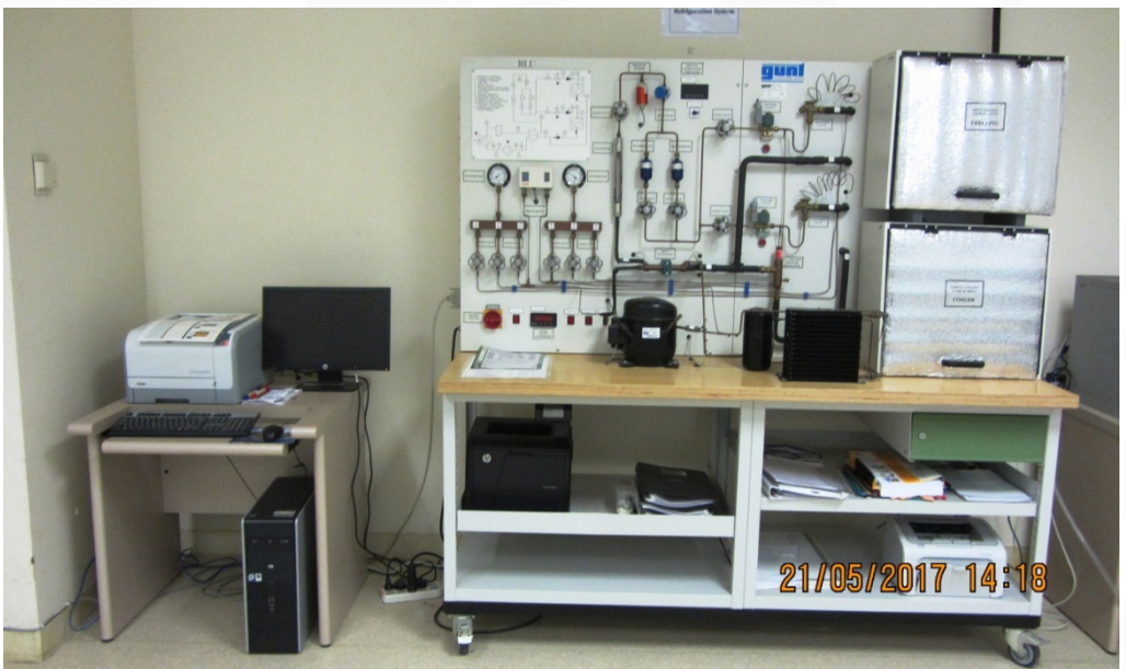
Figure 10.3 Experimental refrigeration multi-pressure vapor compression system.
