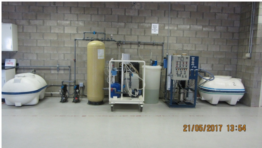
Figure 12.10 Reverse-Osmosis water desalination unit (local department consumption), which can be used as test-rig.
