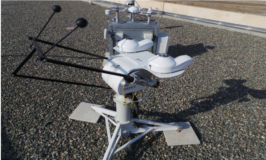
Figure 14.8 Main solar tracking & fixed sensors of KACARE meteorological station for measuring global, direct, diffuse, and normal incidence solar radiation intensity.
