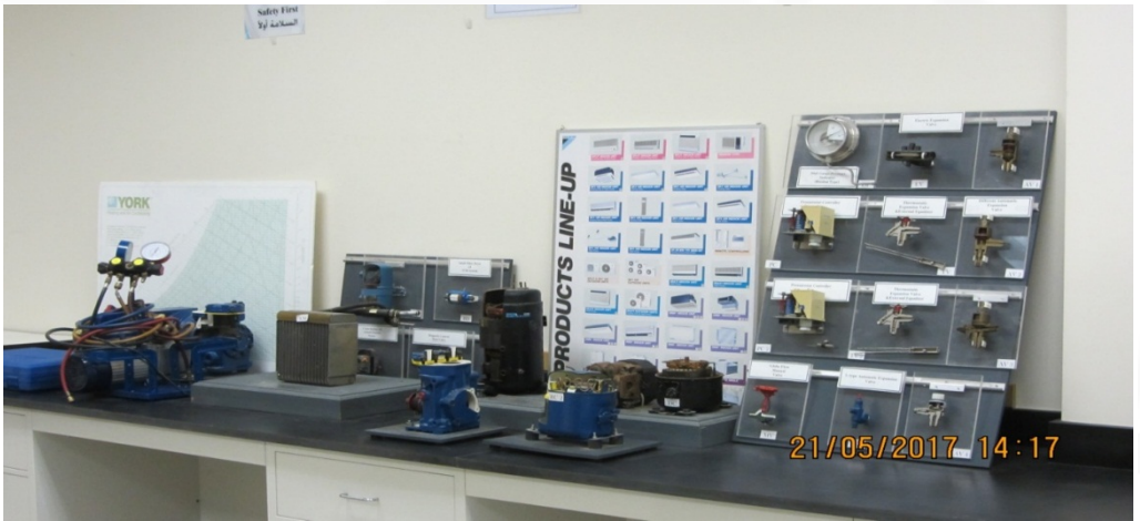
Figure 10.2 Different refrigeration component cross-sections demo units.
