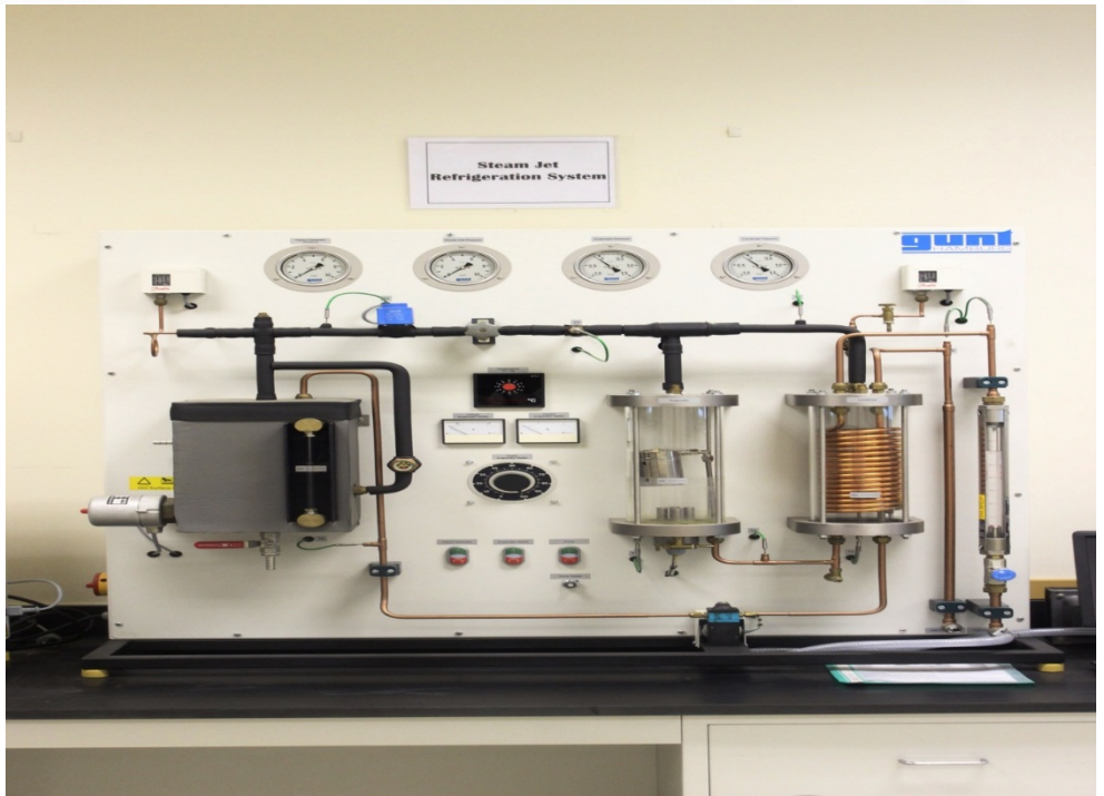
Figure 10.8 Experimental steam-jet refrigeration system.
