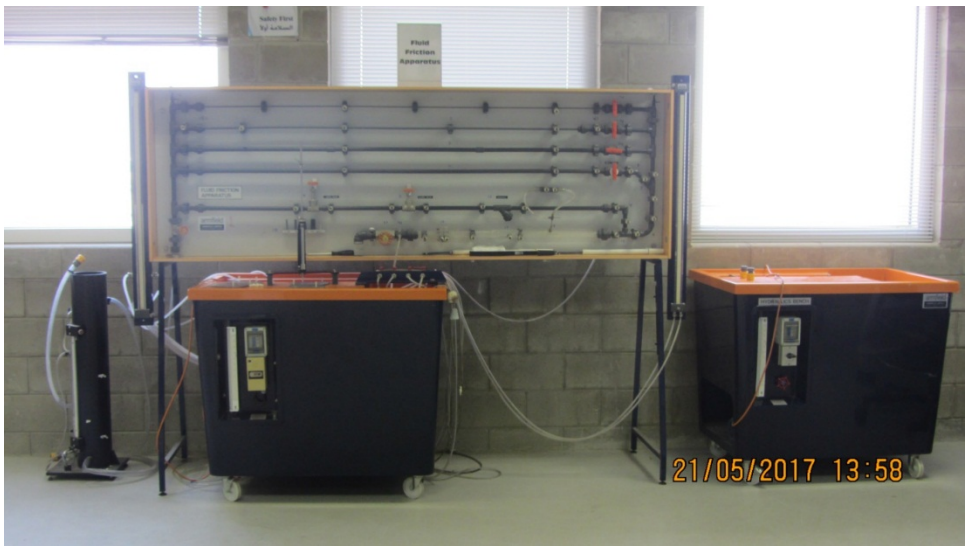
Figure 12.7 Friction loss measurement through pipes, using main circulation water tanks.
