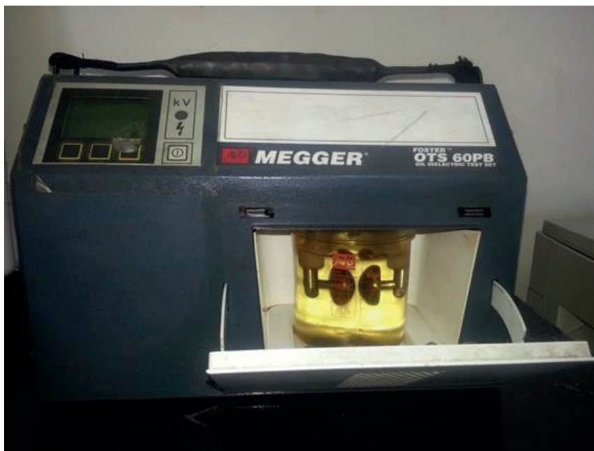
Figure.1 Picture of the device used to measure the breakdown voltage.
