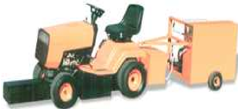
Fig.7 (b) Mobile Microwave Drying- and curing device (Traveling Wave Applicator)
