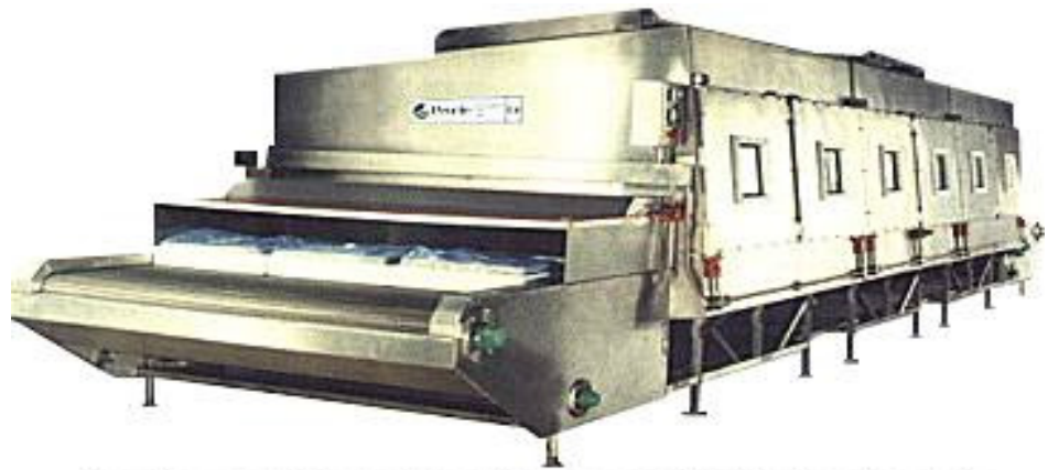
Continuous RF machine thawing 1,000 kg/hr of poultry
