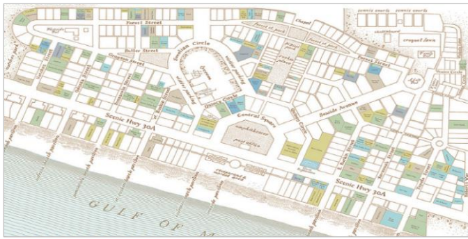
Figure 3 A figure of seaside explains the idea of distributing civil services near homes while minimizing the size of the streets and focusing on pedestrians to access urban services [11].
