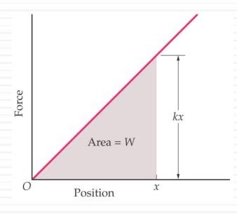
$$W = \int_{x_1}^{x_2} F(x) dx = \int_{x_i}^{x_f} kx dx = \frac{-1}{2} kx_f^2 - \frac{1}{2} kx_i^2 = -\frac{1}{2} kx^2$$
