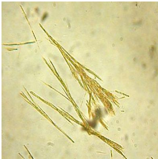
Yellow on heating (Needle shape)
