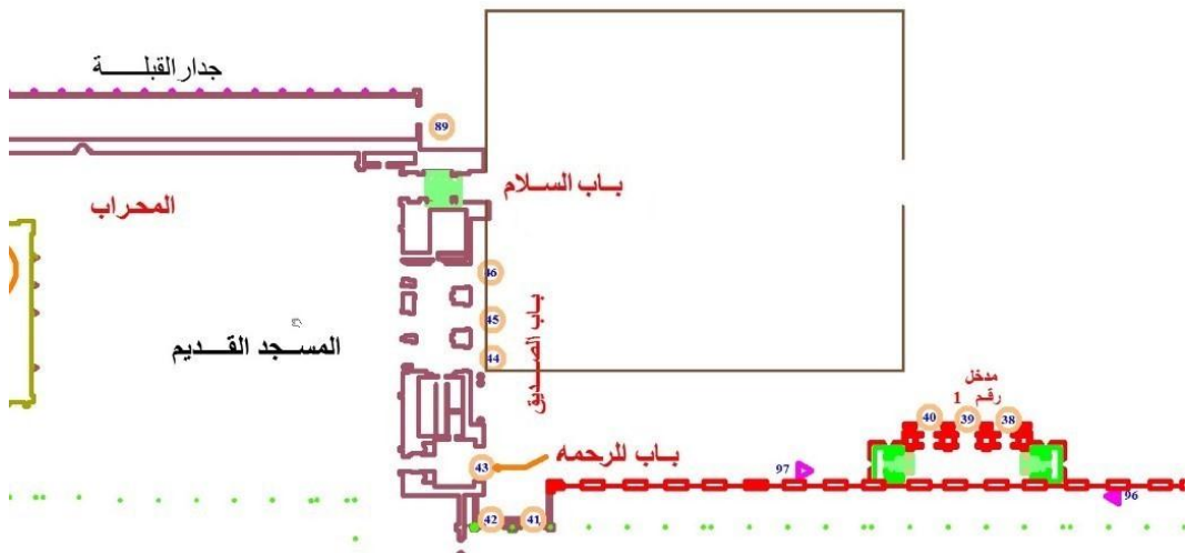
Fig. 1: The fence that is put around El-Salam gate site for controlling crowd flow.
