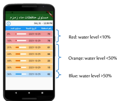
Figure 5: The dashboard mobile app designed for this system as displayed on the device emulator.
