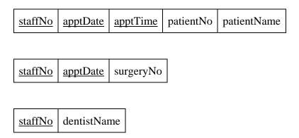
Finally in 3NF we must remove the transitive dependency. In this case we remove the FD3 by splitting into a new table. The transitive dependency left is the patientName that depend on the patientNo, so we split this into new table while creating a foreign key.
