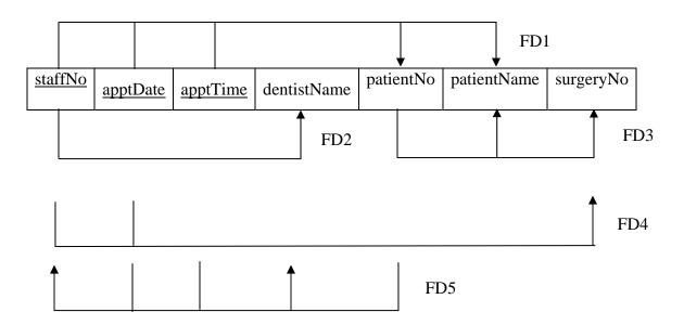
FD1 is already in 2NF. In this case, we can see that FD2 (just depend on staffNo) and FD4 (just depend on staffNo and apptDate) violate the 2NF. These two NFs are partially dependent on the candidate keys not the whole keys. FD2 can stand on its own by depending on the staffNo and meanwhile FD4 also can stand on its own by depending on the staffNo.
