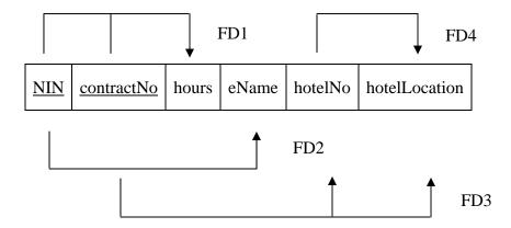
Obviously FD2 and FD3 violate the 2NF (partial dependency) and FD4 violate 3NF (transitive dependency). In the 2NF we remove the partial dependency of the FD2 and FD3 by splitting it into new tables as shown below.
