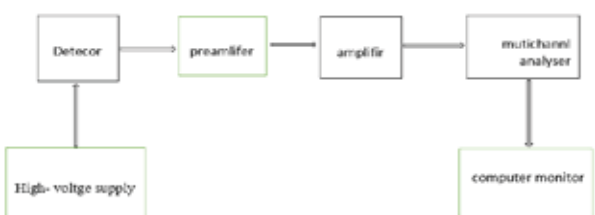
Fig. 3. a schematic electronic system for gamma spectrometry.
