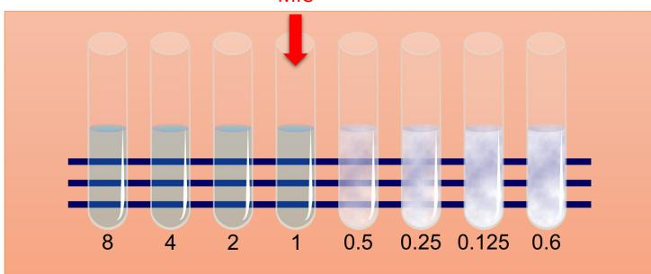
In this figure, the lowest concentration that inhibit the growth of bacteria is 1 ug/ml.
