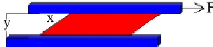
Figure 1.2: Fluid element after the application of a force acting tangentially on the top of the element.
