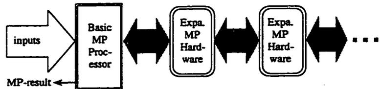
Figure 4.12: The expandable MP system
