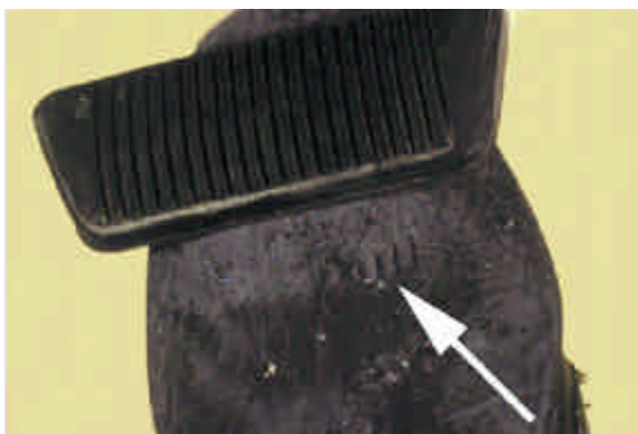
FIGURE 13.5 Leather sole shoes may have impressions from the brake or accelerator pedals. This may give a clue as to how the driver was reacting at the time of the accident.
