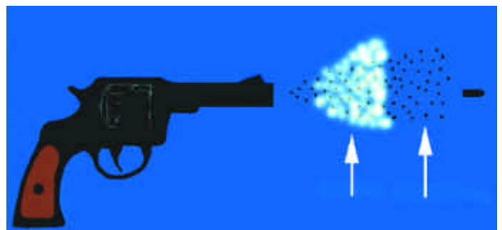
FIGURE 6.4 Gunpowder exits the muzzle in two forms. 1) completely burned powder (soot or fouling) and 2) burning and unburned particles (stippling or tattooing). The particles will travel further than the soot and will abrade the skin.
