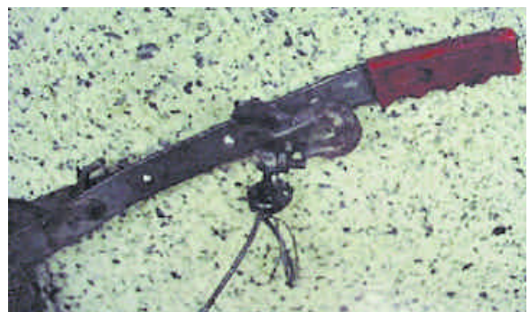
FIGURE 9.28 This is a come-a-long. It is used to move a heavy object toward another object. One end is attached to a support and the hook is attached to the object to be moved. See next photo.
