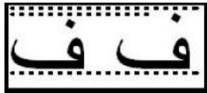
Fig. 2. Shifting the letter "Fa'a" point up to hide bit value equals 1
